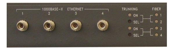
There are two 'TRUNKING' leds, and two pushbutton switches immediately to the left of the 'FIBER' status leds. These indicate and enable/disable trunking or 'link aggregation' for the fiber port 1/2 pair and the port 3/4 pair.
