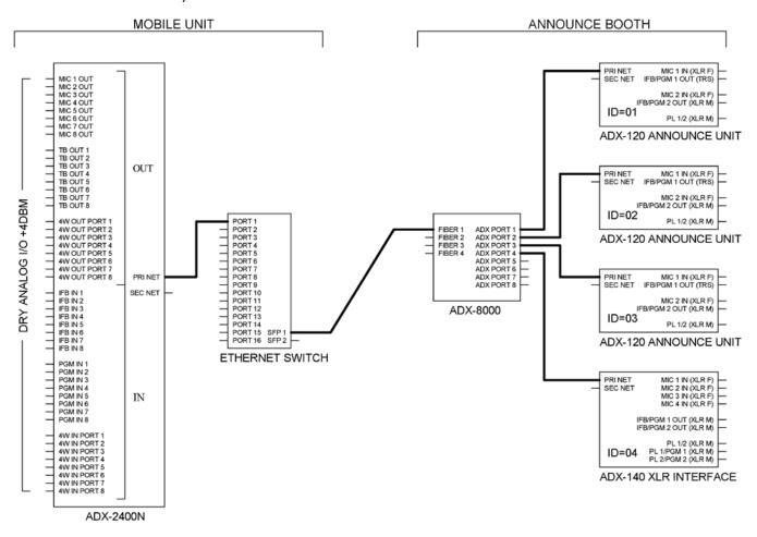
The network connections are very simple and straight-forward. The ADX-2400 in the mobile unit is connected to a generic gigabit switch, such as a Netgear GS716.
