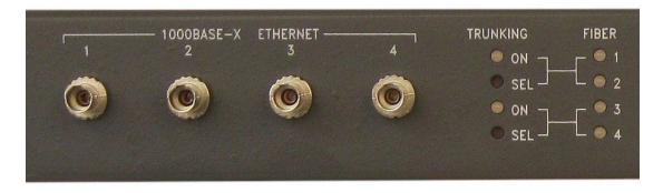
There are four ST connectors which are single-mode, bi-directional gigabit ethernet fiber ports. These panel-mounted ST connectors are connected internally to industry-standard SFP modules.
