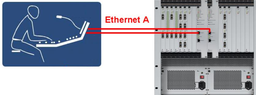
Use a straight (1:1) network cable (STP-CAT 5 with RJ45 connectors):
