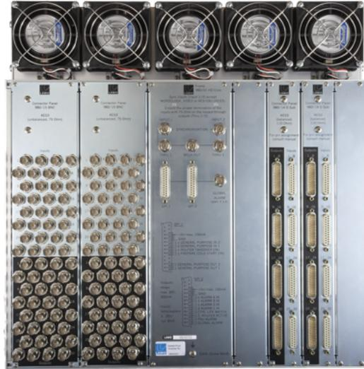
Optionally, the **Nova73 HD** may be fitted with D-Sub and/or BNC AES3 rear connector panels. These provide connections for any [front](#)-mounted AES3 modules (of type 981/02). The two panel types may be mixed allowing up to 8 rear connector panels:
