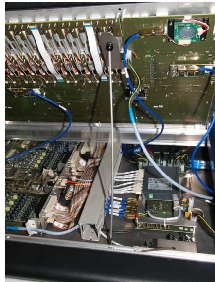
3. When you have completed your service procedure, replace the fastener safely back into its catch, before lowering the central panel.
