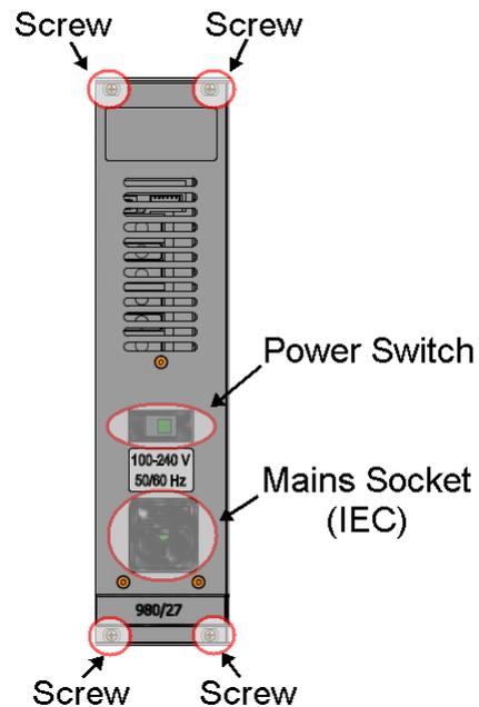
1. Switch off the PSU you wish to replace from the front of the frame as shown above.
