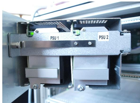
4. Unfasten the metal catch which holds the PSUs in place by pushing on the catch as shown:
