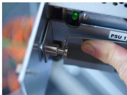
5. Remove the relevant power supply unit and replace with the spare.
