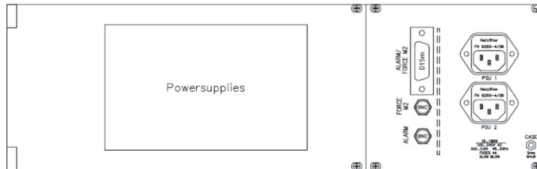
The I/O capabilities of the system are expanded by adding **DALLIS** unit(s). Each may be either 3RU (shown above) or 6RU in height, and may be remote from the rest of the system.
