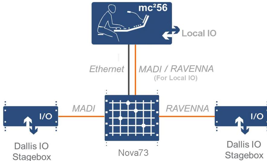
The control system resides on the Router Module MKII (980/33) within the Nova73. Therefore, the following essential connections are required to boot and test the system:
