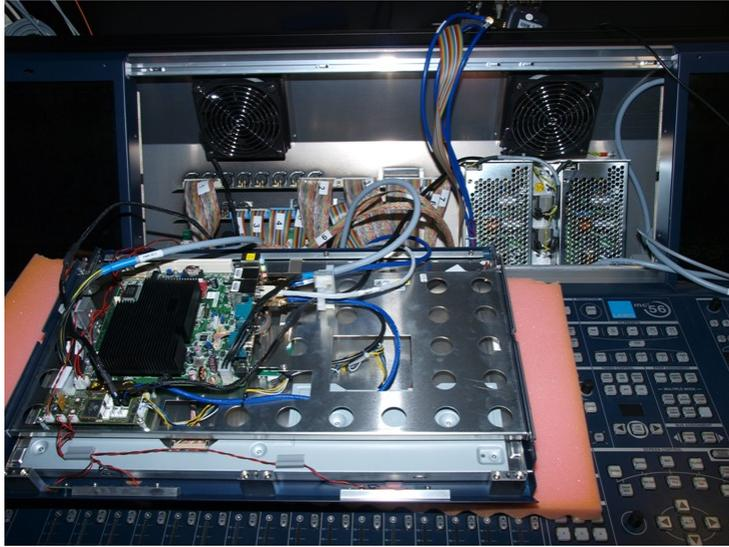
3. Remove the LVDS, USB and power connectors taking notes on where each one should be fitted.
