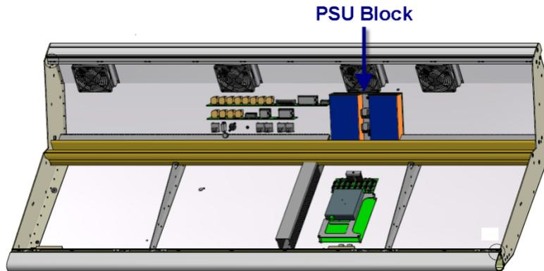
For larger frames, the second PSU block is fitted to the left-most channel bay:
