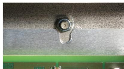
5. Carefully remove the carrier by sliding it forwards and out of the console frame. Take care that the frame does not scrape the unit, and that the cables do not get caught:
