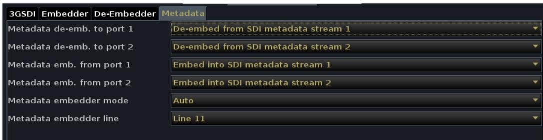
The SDI module offers 2 metadata ports according to SMPTE RDD-2008. This allows embedding, de-embedding and transport of two independent Dolby metadata streams alongside with the video. The streams can be accessed via two D-Sub connectors at the front panel.
