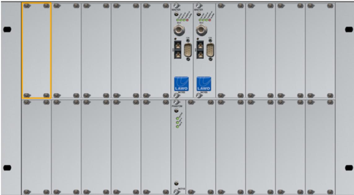
18 double width DALLIS I/O card slots, plus a single width slot reserved for Phantom Power, are available within the [6RU](#) frame. Double width I/O cards (8GU) occupy the whole slot; single width I/O cards (4GU) must be fitted on the left of the slot and a dummy plate fitted to the right to close the gap.
