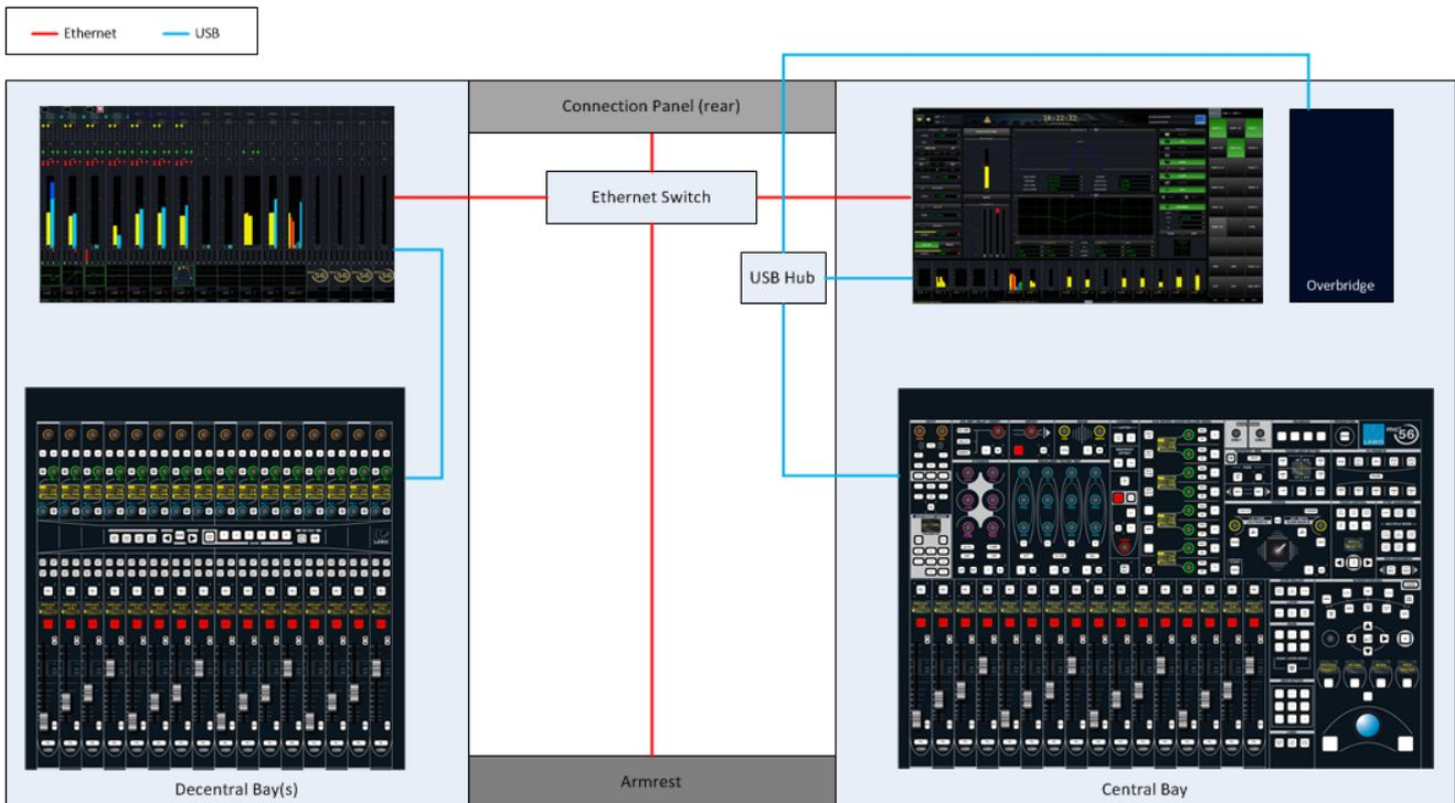
Within each channel and central bay, individual panels and displays connect to an Ethernet Bay Server. (Control surface panels via USB; displays via LVDS for high resolution graphics and USB for touch control).
