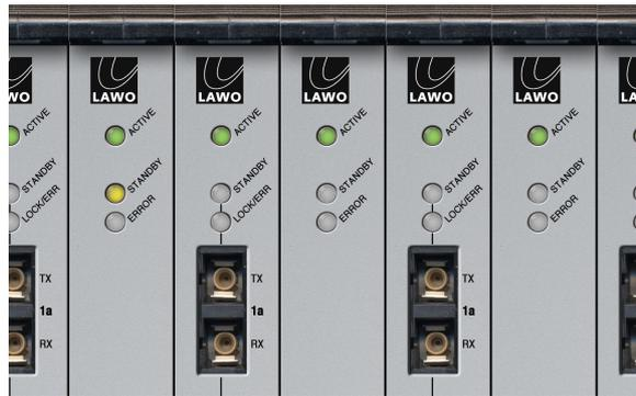
Within the Nova73 a DSP board may be reserved to provide redundant processing (indicated by the **STANDBY** LED).
