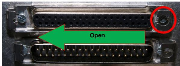
4. Once all the cables have been disconnected and carefully stowed, loosen the local I/O carrier from the console frame. There are two nuts, one at the front (near the console arm rest), and one at the rear (below the Overbridge).
