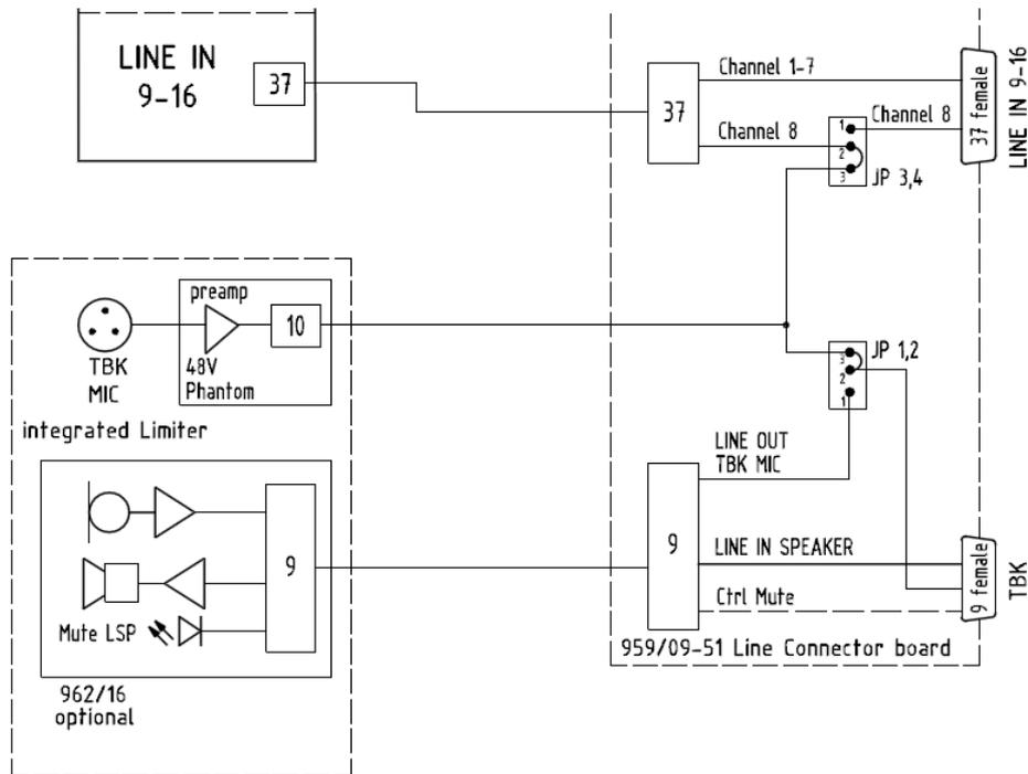
There are four jumper switches on the [local I/O connector board](#), which control two settings:
