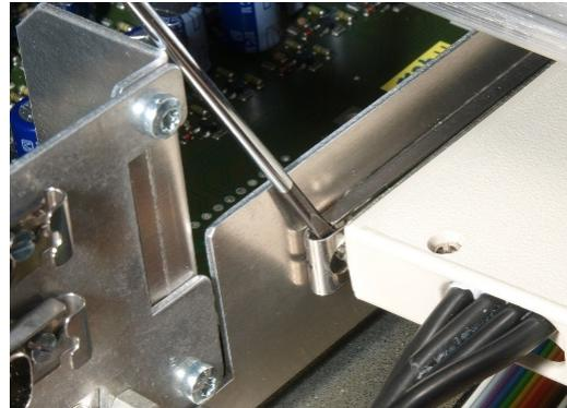
There are two versions of the I/O carrier in the field, using different directions for the sliding lock mechanism. You can verify the direction by looking at the position of the screws; when open, the screws are not covered by the sliding part:
