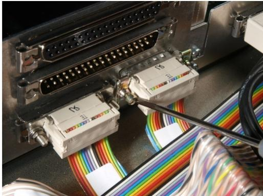
**D-Sub Sliding Lock Mechanism**
