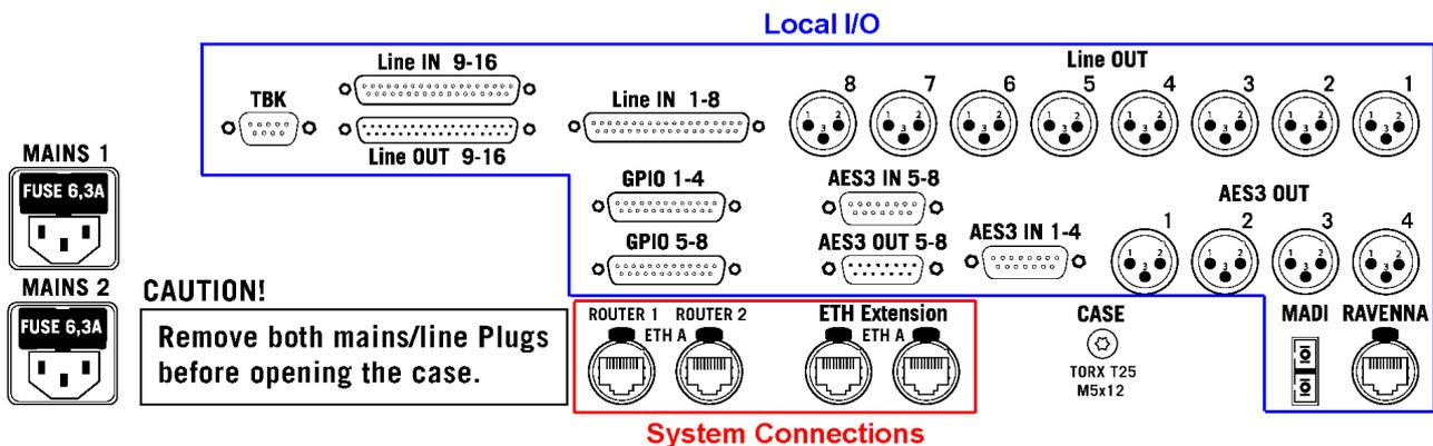
It is recommended that **MAINS 1** and **MAINS 2** be run from separate phases of the mains supply, and that the same two phases are used for all parts of the desk. It is also recommended that all power connections are controlled from a common mains switch.
