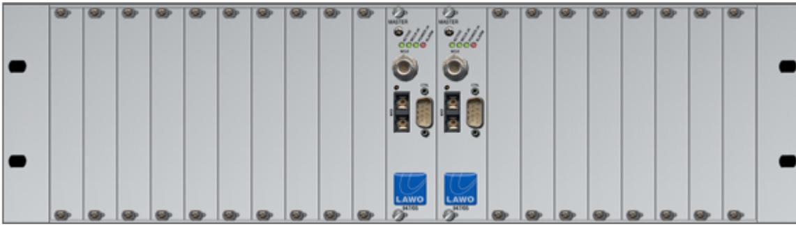
18 single width DALLIS I/O card slots are available within the [3RU](#) frame. Double width I/O cards (8GU) occupy two slots; single width I/O cards (4GU) occupy one slot.
