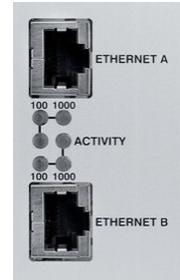
Connections are made via TCP/IP Ethernet.
