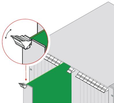
This unlocks the module from the Nova73 and automatically disables it; the module's LEDs should be off. Note that it is not necessary to pull out or remove the module.
