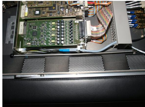
2. Release the fastener from its catch, and position it against the metal plate (to the left of the trackball) as shown:
