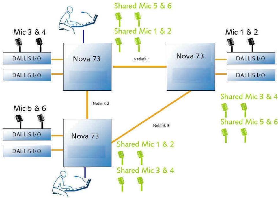
In the example above, mics are physically connected, via a DALLIS, to each system. Signals are transferred between systems via 'Netlinks', providing the ability to share any mic input.
