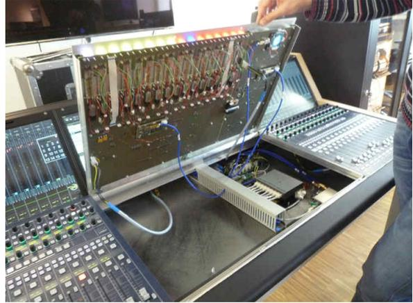
4. Carefully remove the panel by lifting it out of the frame.
