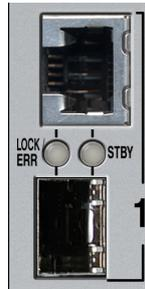
2. Press gently and firmly until the module locks into position.
