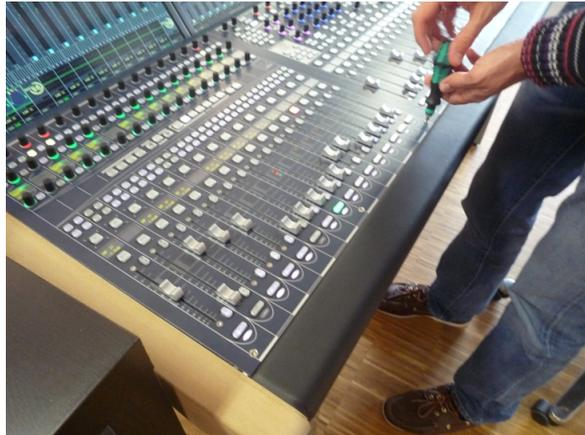
You should remove the screws completely and place them carefully to one side, so that they do not fall into the frame when the panel is lifted. The springs beneath the panel will raise it slightly from the frame.
