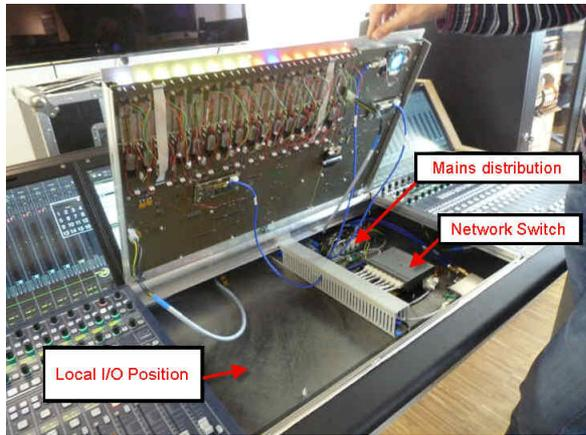
Local I/O Carrier Unit (disconnected)
