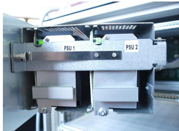
Depending on your system specification, each DALLIS may be delivered with single or dual redundant power supply units (PSUs).
