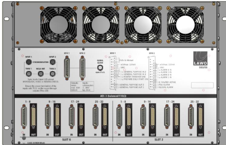
The [Nova73 Compact](#) comes with rear-mounted AES3 connectors as standard. These provide balanced 110  $\Omega$  D-Sub connections for up to two front-mounted AES3 modules (of type 981/02). Note that the AES3 modules *MUST* be fitted to slots 2 and 6 at the [front](#) of the core.
