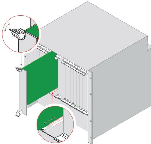
*When fitted correctly, it will lock into place.*
