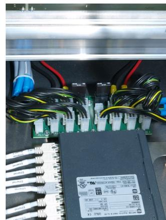
3. Using a T20 Torx driver, disconnect the PSU block from the distribution board by removing the 4 wires shown below:
