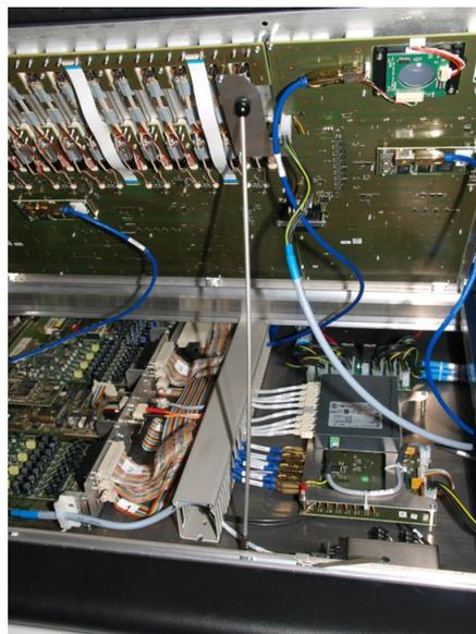
3. Remove all of the connectors from the local I/O carrier, in the order described below, taking notes on where each one should be fitted:
