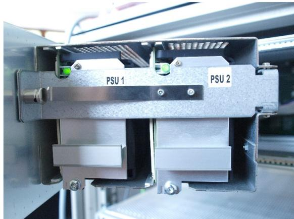
The Nova73 HD, Nova73 Compact and DALLIS provide two slots for dual redundant power supplies, see [Nova73 power](#) and [DALLIS power](#). Their status may be monitored from the console GUI using the [Signal Settings](#) display.
