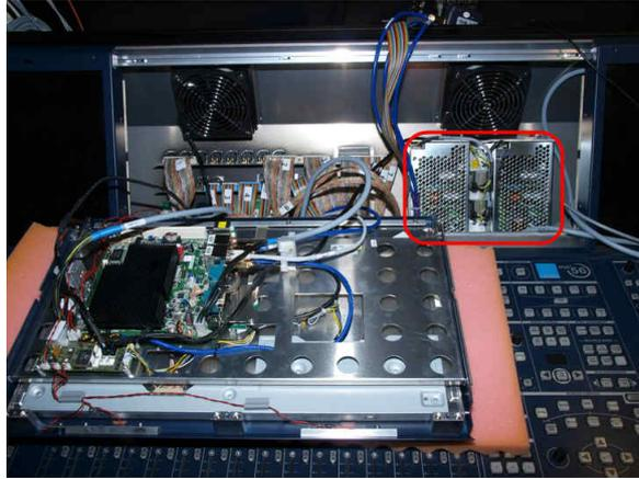
6. Using a 7mm hex socket, remove the two screws holding the power supply block in place, followed by the single screw attaching the protective earth:
