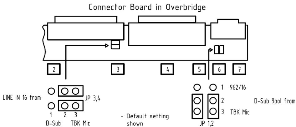
2. Locate the correct pair of jumper switches: either 3 & 4 (**JP 3,4**) or 1 & 2 (**JP 1,2**) - the locations and default positions are shown above and below:
