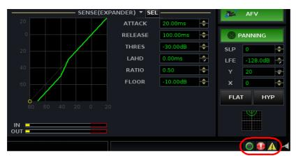
The number of symbols relates to the number of PSU blocks within the control surface and whether any extender bays with their own PSU are fitted. PSU blocks are represented from left to right, and each block consists of two supplies running in parallel.
