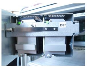
4. Unfasten the metal catch which holds the PSUs in place by pushing on the catch as shown:
