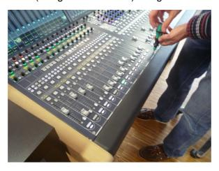
You should remove the screws completely and place them carefully to one side, so that they do not fall into the frame when the panel is lifted. The springs beneath the panel will raise it slightly from the frame.
