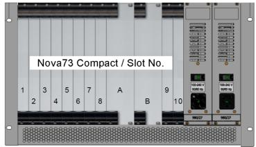
The diagrams above show the front module slots available within the Nova73:
