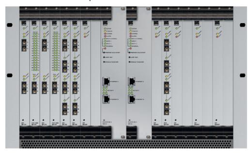
• ACTIVE LED – shows that the module's internal control system is booted and running.
