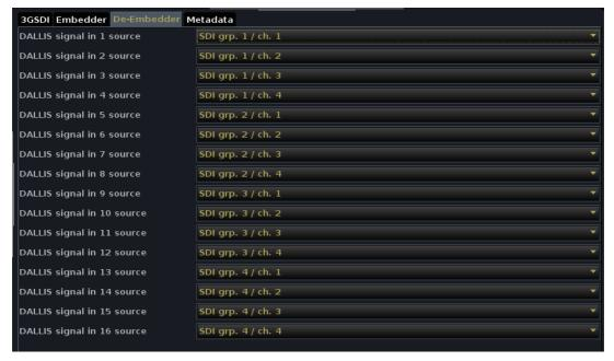
• DALLIS signal in source 1 to 16 – use these options to define the source for each deembedder.
