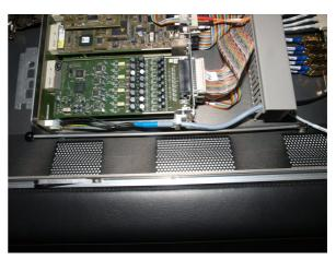
2. Release the fastener from its catch, and position it against the metal plate (to the left of the trackball) as shown:
