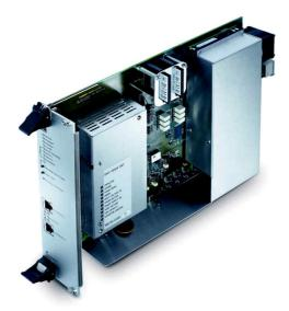
1. Power off the Nova73 (both PSUs if fitted) and remove the Router Module.
