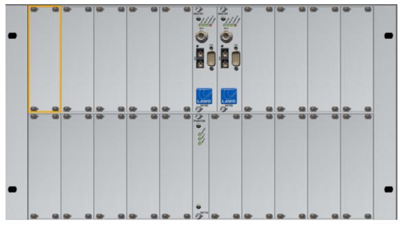
18 double width DALLIS I/O card slots, plus a single width slot reserved for Phantom Power, are available within the 6RU frame. Double width I/O cards (8GU) occupy the whole slot; single width I/O cards (4GU) must be fitted on the left of the slot and a dummy plate fitted to the right to close the gap.
