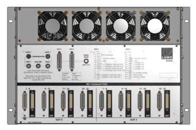
The <u>Nova73 Compact</u> comes with rear-mounted AES3 connectors as standard. These provide balanced 110? D-Sub connections for up to two front-mounted AES3 modules (of type 981/02). Note that the AES3 modules *MUST* be fitted to slots 2 and 6 at the <u>front</u> of the core.
