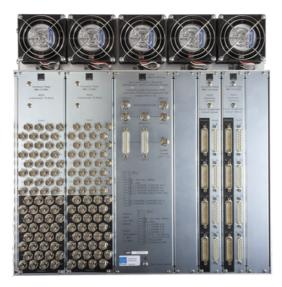
Optionally, the **Nova73 HD** may be fitted with D-Sub and/or BNC AES3 rear connector panels. These provide connections for any <u>front</u>-mounted AES3 modules (of type 981/02). The two panel types may be mixed allowing up to 8 rear connector panels:
