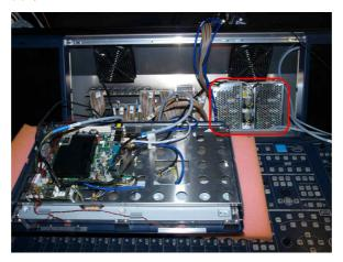
**6.** Using a 7mm hex socket, remove the two screws holding the power supply block in place, followed by the single screw attaching the protective earth:
