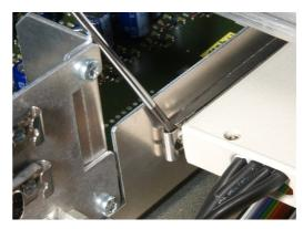
There are two versions of the I/O carrier in the field, using different directions for the sliding lock mechanism. You can verify the direction by looking at the position of the screws; when open, the screws are not covered by the sliding part:
