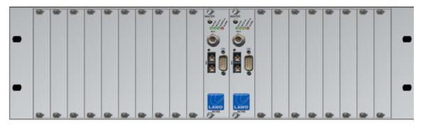
18 single width DALLIS I/O card slots are available within the <u>3RU</u> frame. Double width I/O cards (8GU) occupy two slots; single width I/O cards (4GU) occupy one slot.
