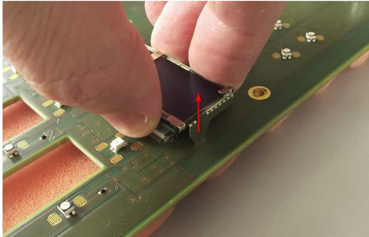
Open the locks and remove the flat foil + OLED:
