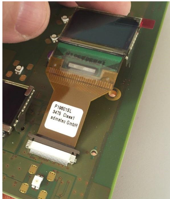
Bring the OLED into its final position while the flat foil will be bent very slowly and clip the holder in its position:
