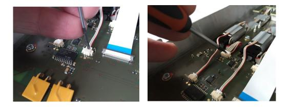
Turn the panel and open all T10 fader screws and remove all fader:
