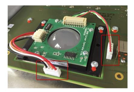
Turn the panel, open the locks and remove the flat foils between the PCBs:
