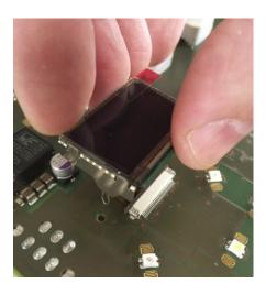
Remove the security plastic film from every single OLED
