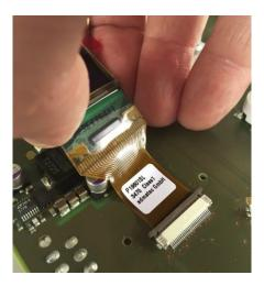
Bring the OLED into its final position while the flat foil will be bent very slowly and clip the holder in its position:
