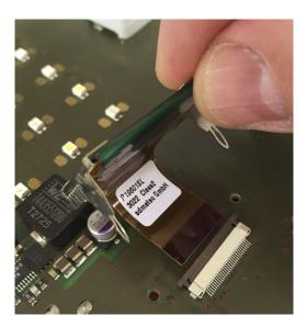
Open the locks and remove the flat foil + OLED:
