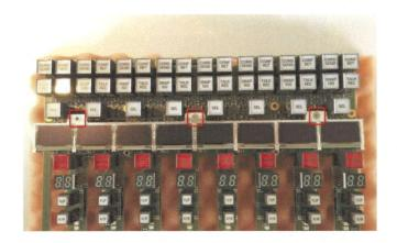
open all flatfoil locks and remove the OLED bar:
