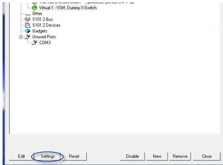
The vsmStudio software allows each port to be adapted individually. To do so, access the window *Manage Communication Ports* through the main menu or by pressing F8. Select the layer to be adjusted and select *Settings*.
