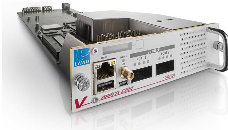
The C100 plug-in cards slot into the front of the V\_\_matrix frame.
