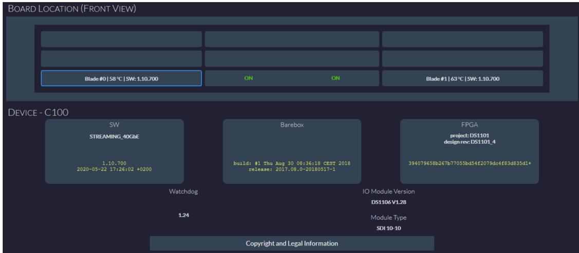
The boxes at the top represent the V\_\_matrix frame slots as viewed from the front. Here you can see the status of the two power supplies and C100 processing blades.
