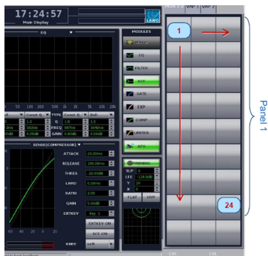
mc256 monitor panel (touch / GUI)
