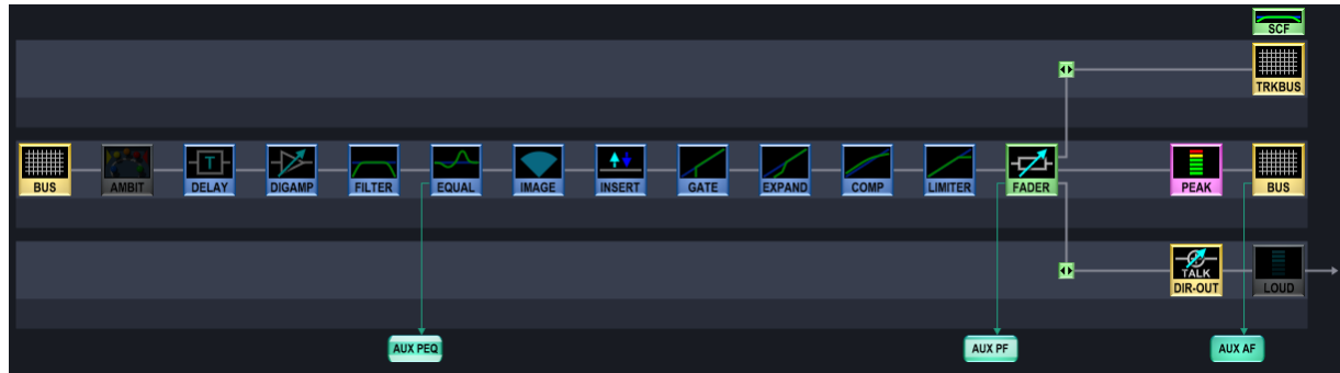
Group Channel (Recording channel DSP Configuration)
