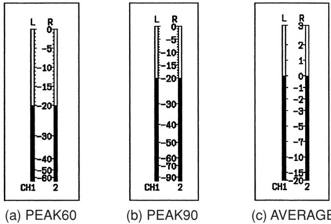
The figure shows the scale when the reference level is set to -20 dB and the scale is set to TYPE-A.
