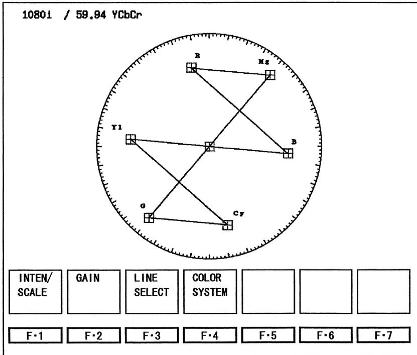
Figure 7.2 Vectorscope display and vectorscope display menu
