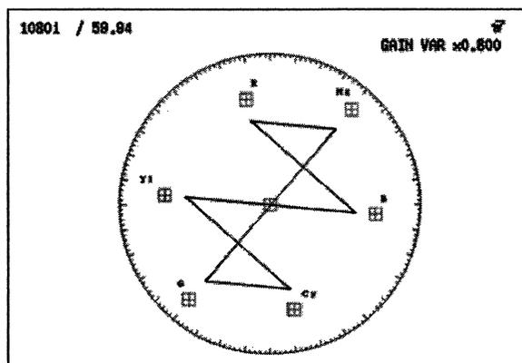
Figure 7.6 Gain Variable Display
