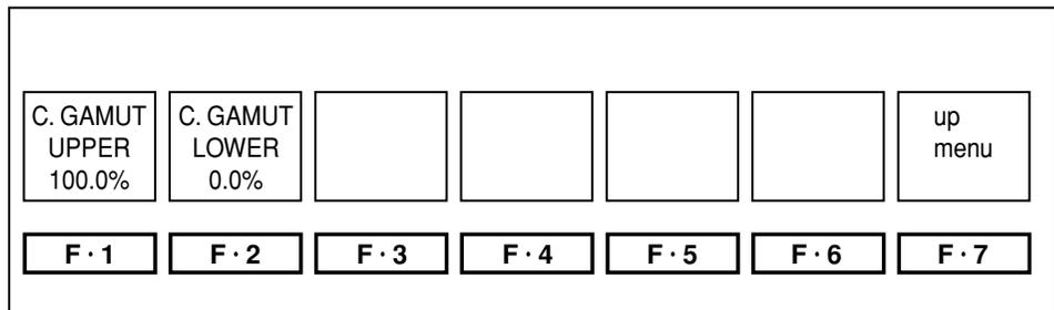
Figure 11.18 Composite gamut error threshold level setup menu
