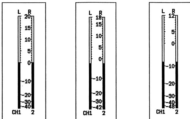
Figure 9.9 TYPE-B level meter according to the reference level
