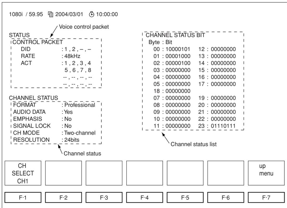
Figure 11.11 Detailed status display of embedded audio
