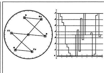
(b) Waveform display and vectorscope display
