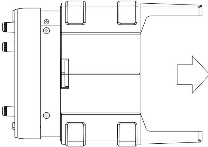
Figure 3.5 Direction for removing the case (side panel)
