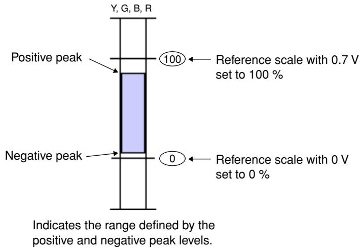
Figure 14.5 Bar display contents of component signal
