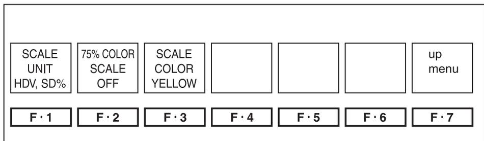
Figure 6.20 Scale Setup Menu
