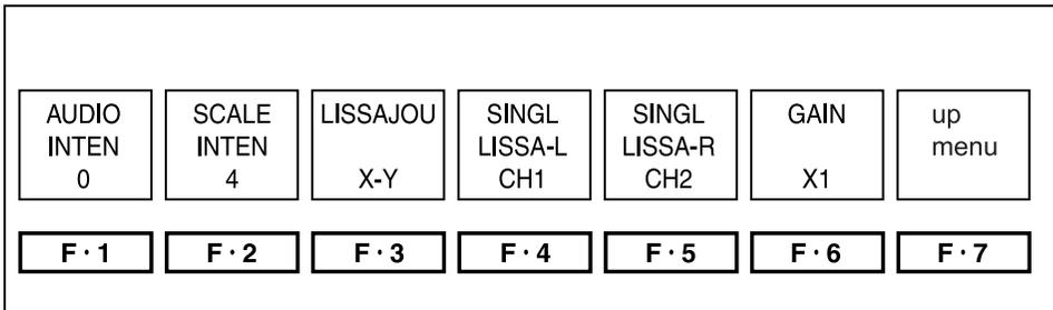
Figure 9.4 Audio waveform display menu
