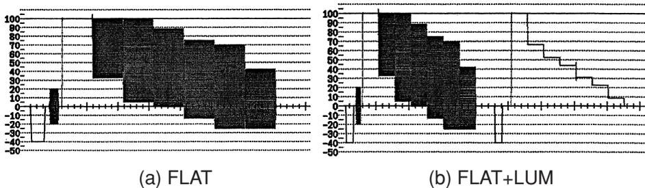
Figure 6.10 Filter Waveform of the Pseudo-composite Display
