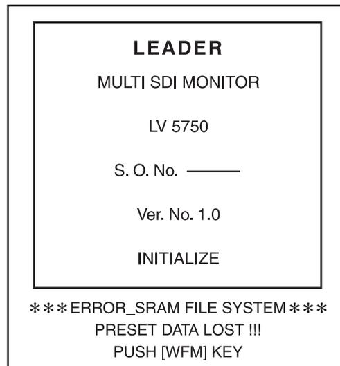
Figure 1.2 Message that appears when the backup battery runs out
