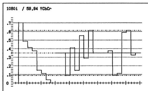
Figure 6.22 75 % Color Bar Scale
