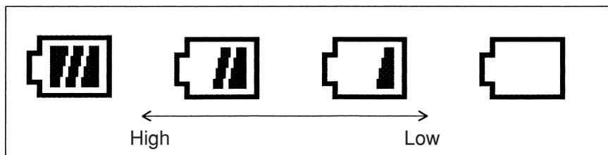
Figure 14.2 Remaining battery power display
