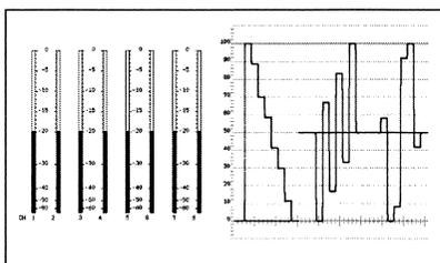
(e) Waveform display and audio level display
