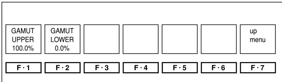
Figure 11.17 Gamut error threshold level setup menu
