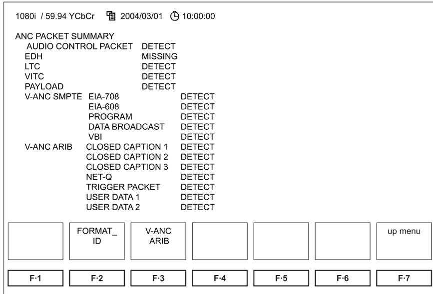
Figure 14.8 ANC Packet Detection Display and ANC Packet Menu
