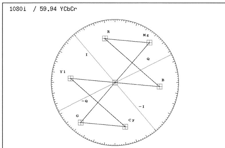
Figure 7.4 IQ axis on the vectorscope display
