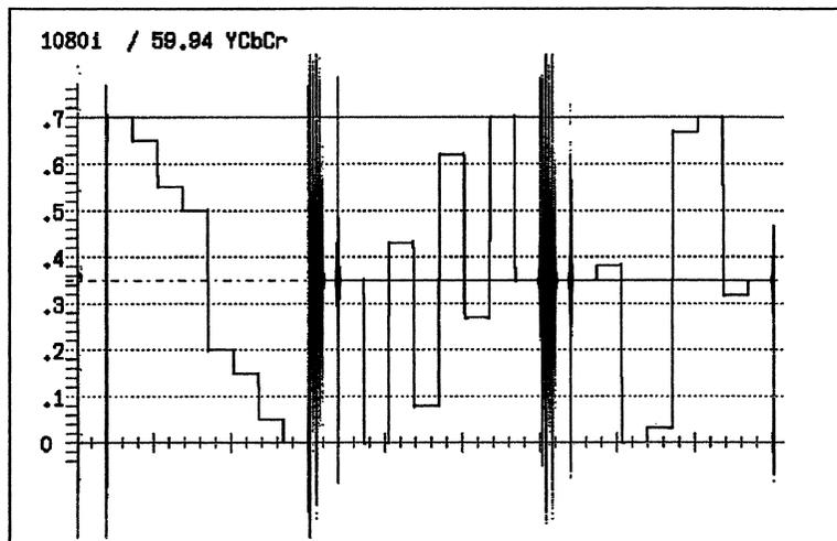
Figure 6.23 Waveform Display during the Blanking Period
