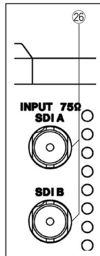
Figure 5.1 SDI signal input connectors ②⑥ (INPUT SDI A,B)
