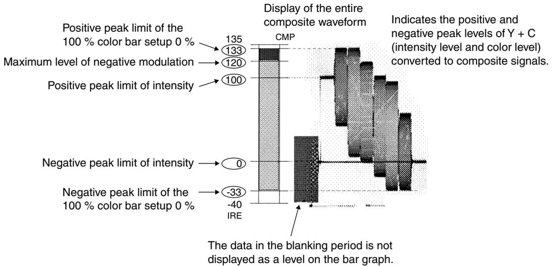
Figure 14.6 Bar display contents of composite signal
