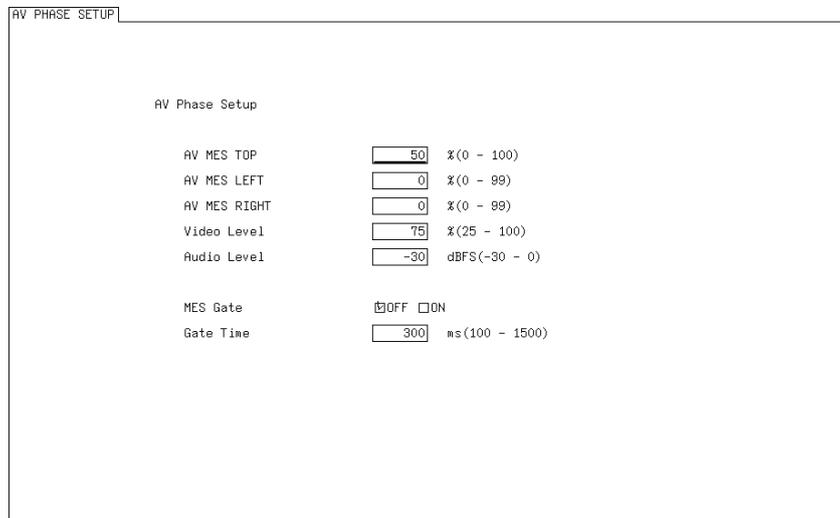
Figure 6-16 AV PHASE SETUP tab
