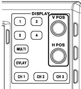
Figure 2-3 V POS and H POS knobs
