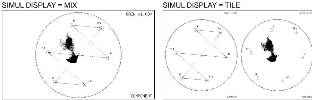
Figure 3-11 Setting the simul display
