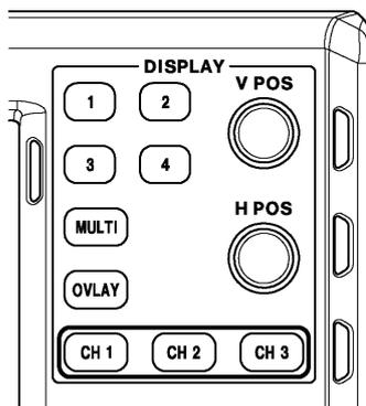
Figure 2-6 The CH1 to CH3 keys
