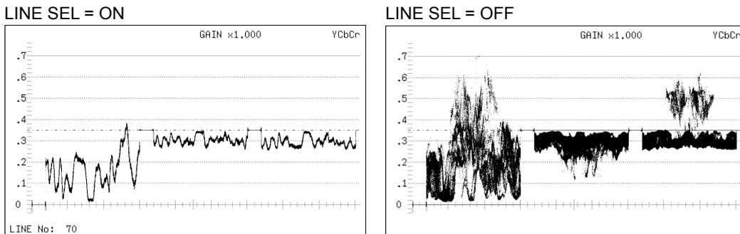
Figure 2-21 Turning line select on and off
