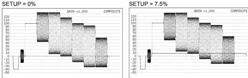
Figure 2-33 Selecting the setup level
