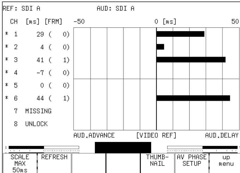
Figure 6-14 Lip sync measurement screen
