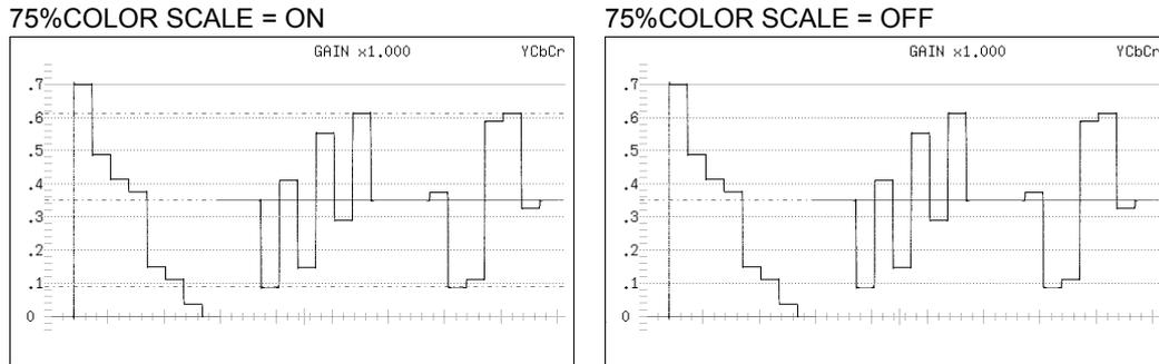
Figure 2-10 Displaying a scale for 75 % intensity color bars
