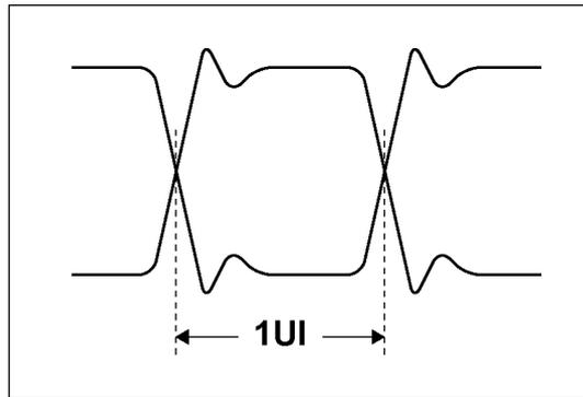
Figure 7-7 Unit interval
