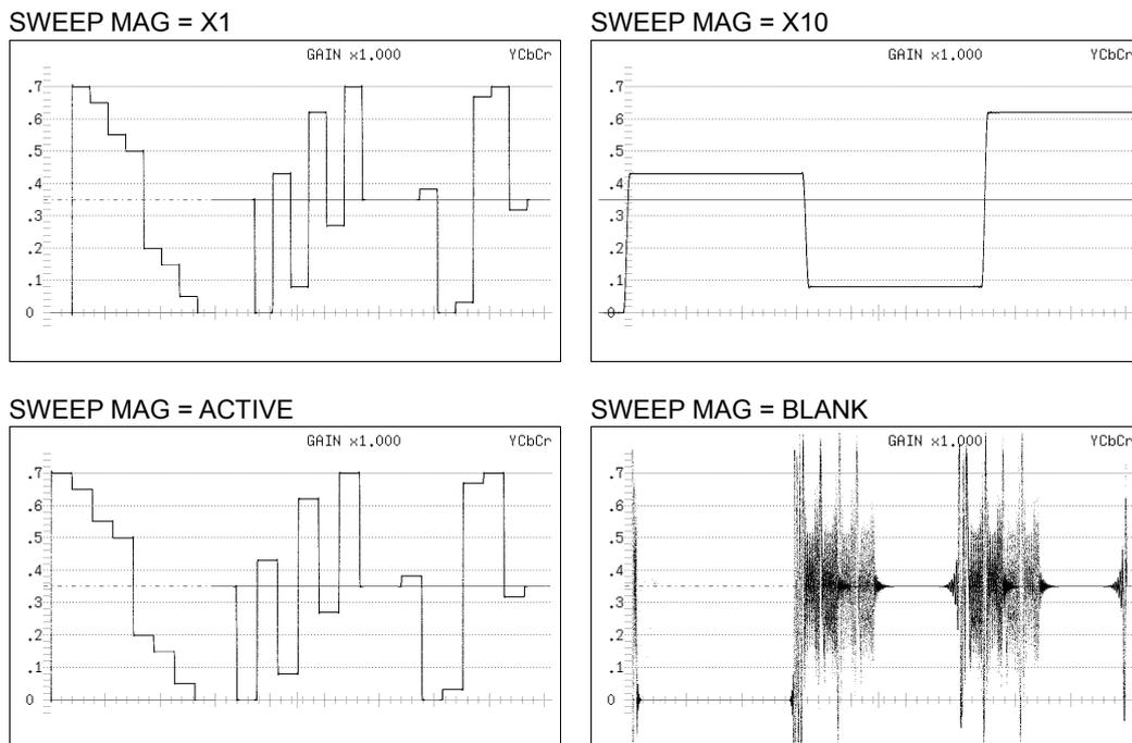
Figure 2-18 Horizontal magnifications
