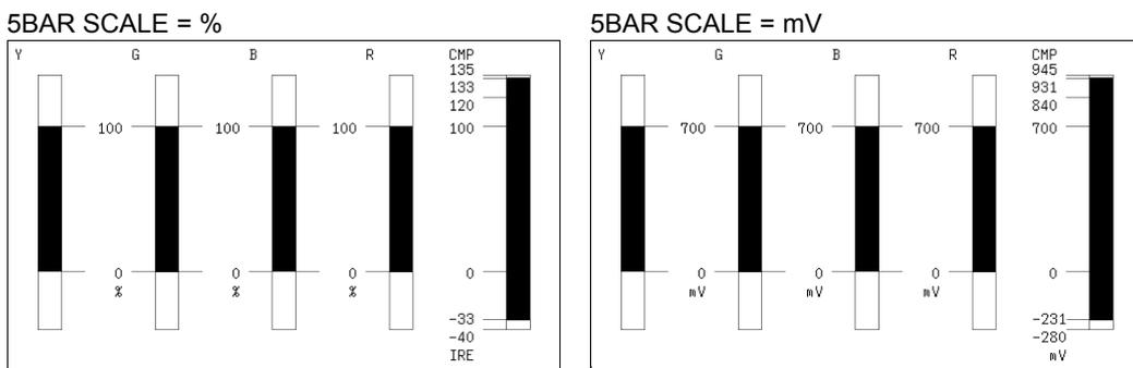
Figure 3-21 Selecting the scale unit
