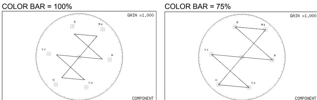
Figure 3-18 Displaying a scale for 75 % intensity color bars (when receiving a 75 % intensity color bar signal)
