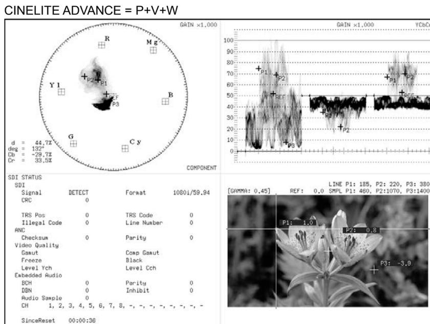
Figure 4-18 Displaying synchronized markers
