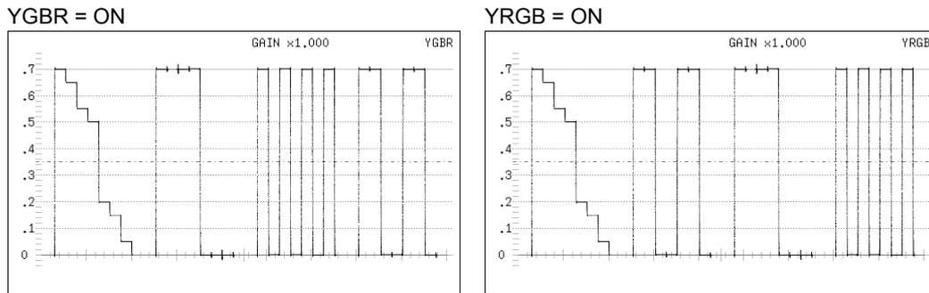
Figure 2-31 Turning the luminance signal on and off
