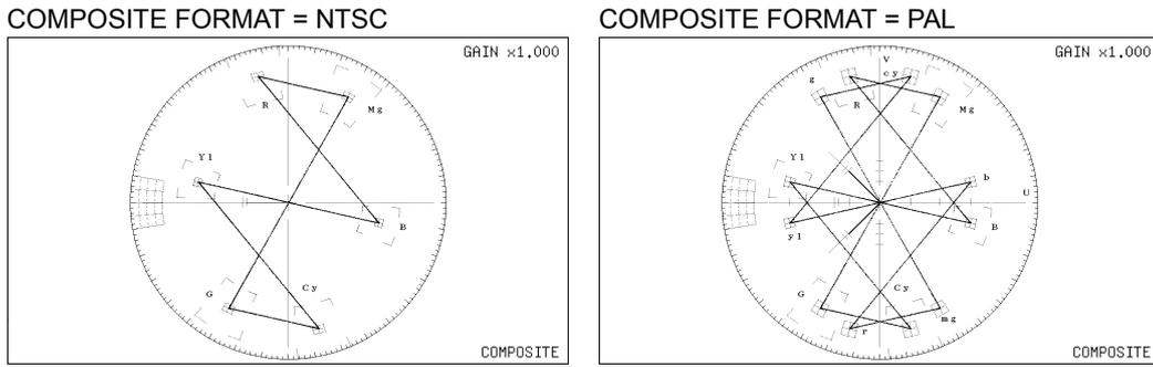
Figure 3-17 Selecting the composite display format
