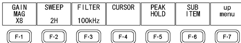
Figure 7-16 JITTER SETUP menu
