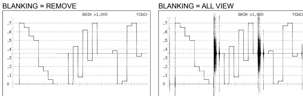
Figure 2-19 Displaying blanking intervals
