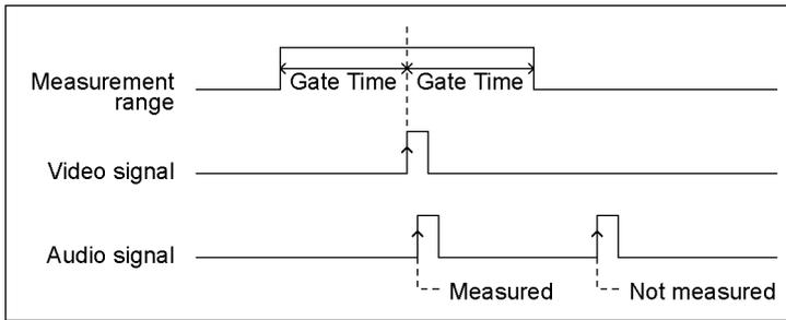
Figure 6-18 Setting the measurement range (Audio signal)
