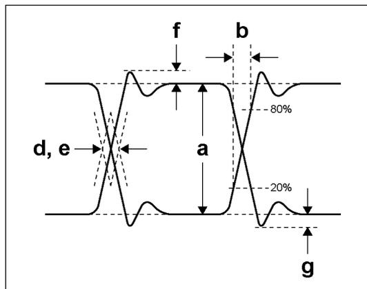
Figure 7-6 Explanation of measurement items
