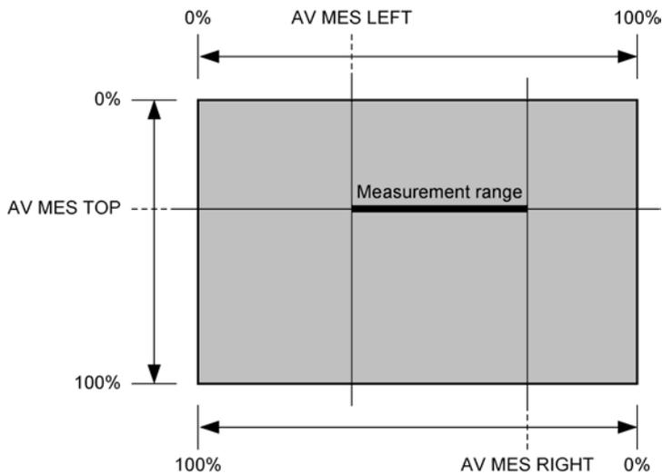
Figure 6-17 Setting the measurement range (Video signal)
