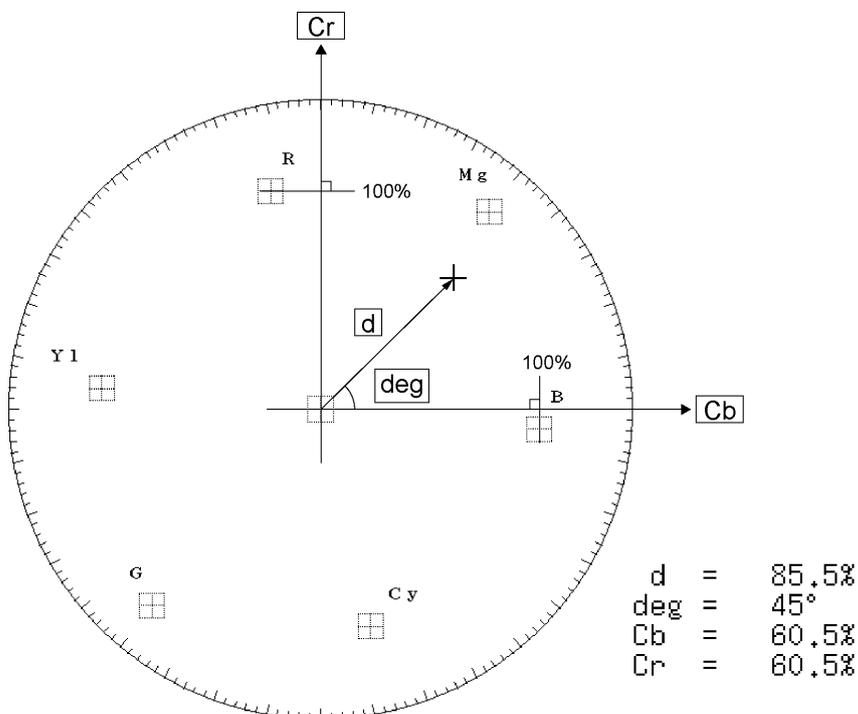
Figure 3-8 Displaying the vector marker
