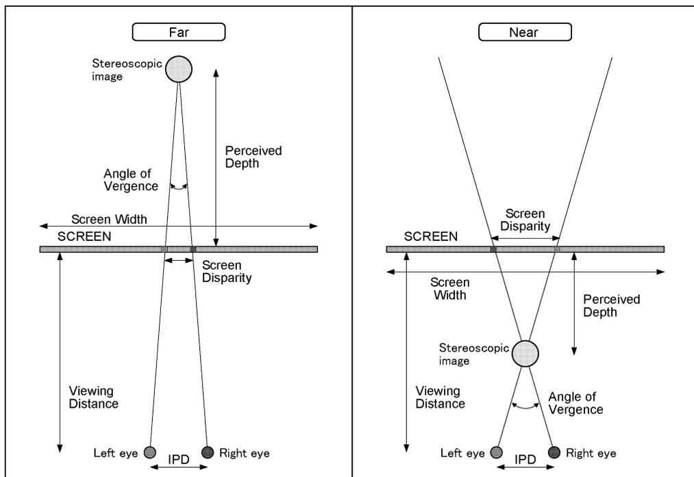
Figure 5-8 Setting and measurement item names
