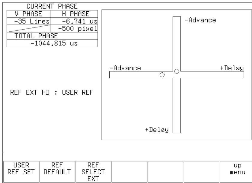
Figure 6-13 Phase difference measurement display
