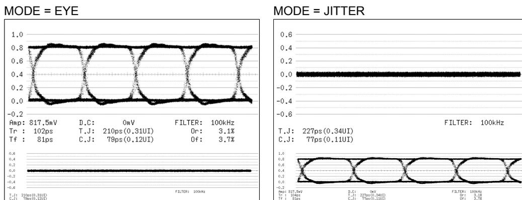
Figure 7-5 Selecting the display mode
