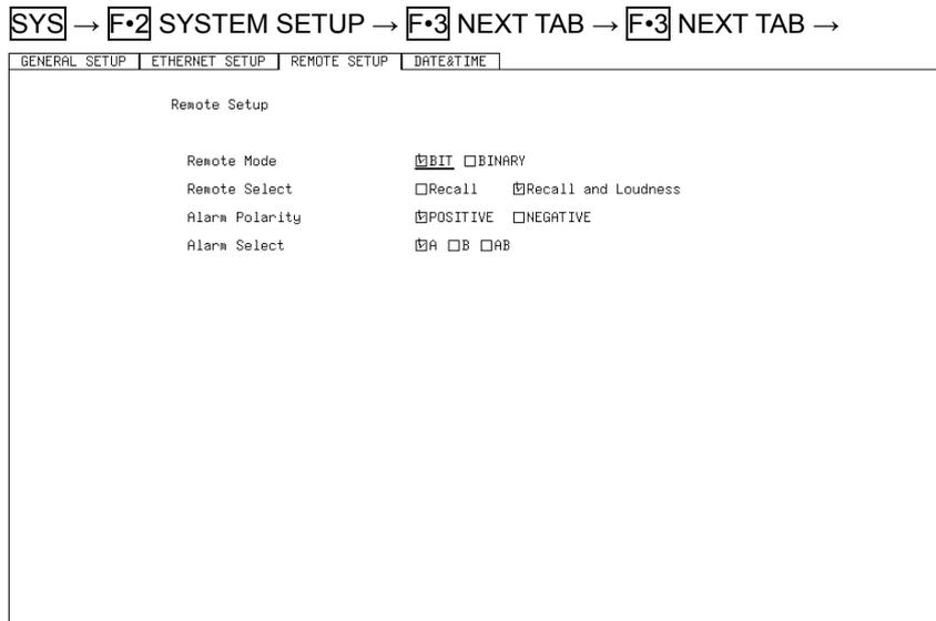
Figure 7-8 REMOTE SETUP tab
