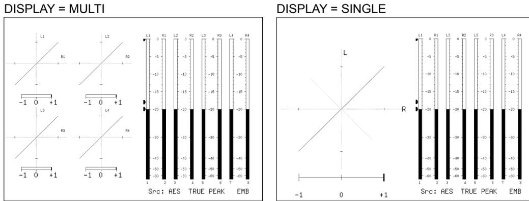
Figure 4-2 Selecting the Lissajous curve display format
