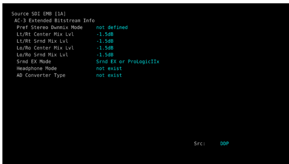
Figure 7-26 Dolby Digital Plus EBI metadata display
