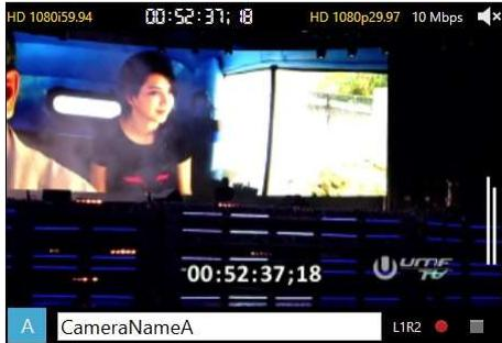
This name will display on the video monitoring window of the channel, and will also be used to generate file names. When a record is started, the corresponding file name will be created as YYYYMMDD\_HHMMSS\_ChannelName.mov, where YYYY is the year, MM the month, DD the day, HH the hour, MM the minute, SS the second, when the record was started. Example of file name : 20150903\_190123\_Camera1.mov.
