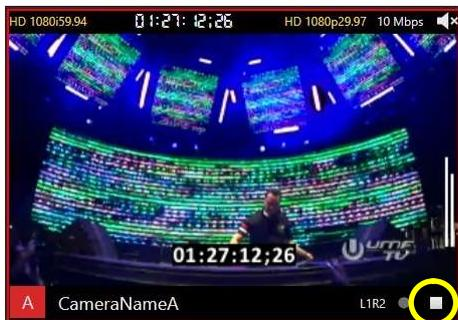
To stop recording all channels at once, use the global Stop button in the lower part of the main window.
