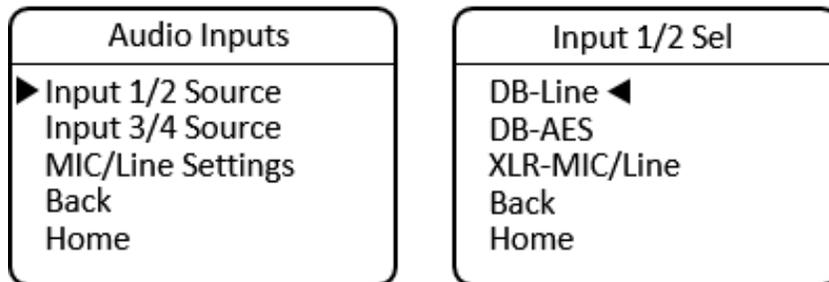
When selecting AES for inputs 1 and 2, the input is taken from the channel 1 input. After setting the source, navigate back one level to configure the settings for input 3 and 4.
