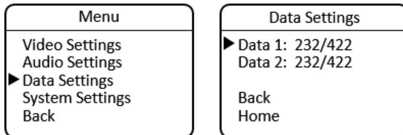
The Camera serial data settings may also be configured remotely, from the webpage dashboard accessed from the Base Unit.
