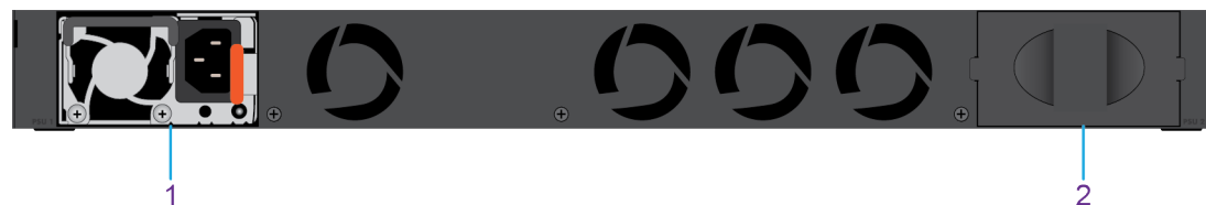
Figure 8. Back panel model M4300-24X24F
