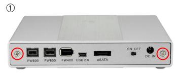
Using a Phillips P0 screwdriver, remove the 2 screws that hold the rear backplane cover to the enclosure.
