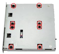
With your fingers holding the drive mechanisms into the enclosure, flip it over onto the top so you can see the screw holes that you will need to use in the next step.
