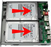
Place your drive mechanisms onto the bridge card, and press the drives towards the ports to firmly affix the drives into the SATA connectors.
