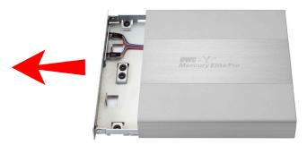
From the rear of the enclosure, press inwards on the rear ports to slide the inner chassis out towards the front of the enclosure.
