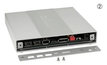
Once the screws are removed, the rear backplane cover will easily come off.
