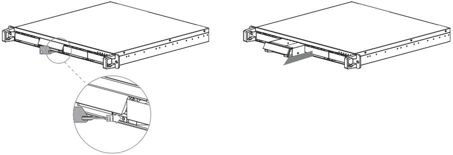
B. Remove the holder from the removable tray with a screwdriver (be careful not to damage the nuts)
