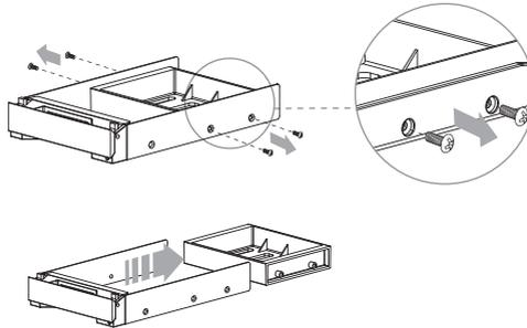
C. Mount the hard disk drive and fasten the screws.
