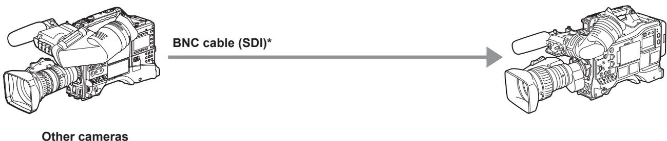
\* For the BNC cable (optional) connected to the <SDI IN> terminal, prepare a double-shielded cable equivalent to 5C-FB.
