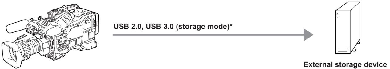
\* The USB 2.0 cable and USB 3.0 cable are not supplied with the camera. Prepare a commercial USB 2.0 cable or USB 3.0 cable (double-shielded for noise suppression).
