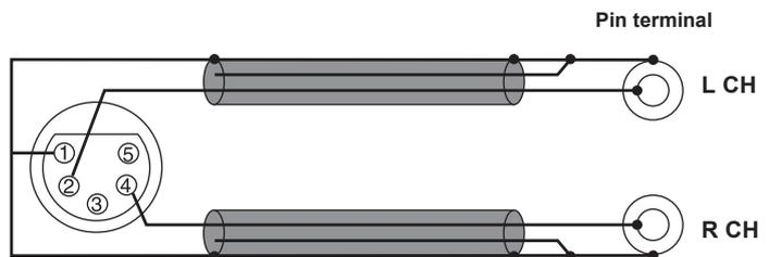
Do not use the cable where the pin 3, pin 5 and pin 1 are connected. Doing so may result in a malfunction.
