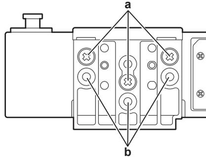
**a:** Normal positions of securing screws
