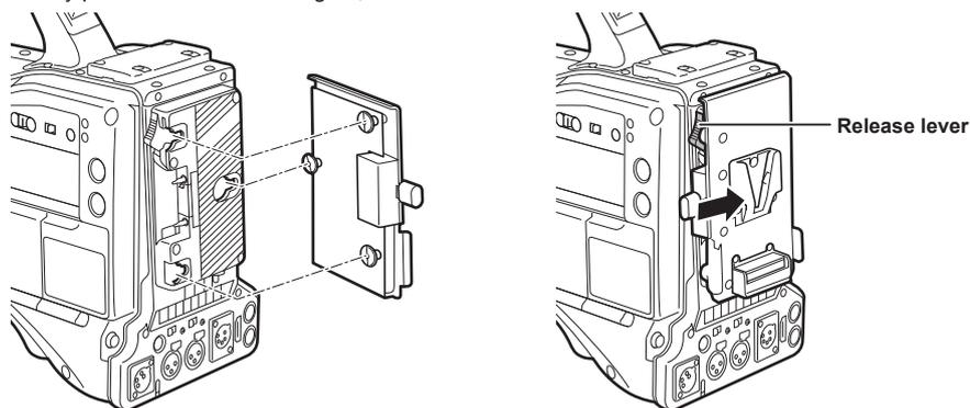
**1** Mount the V-mount type battery plate.
