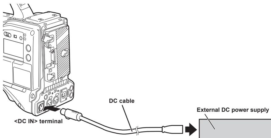
**1** Connect the external DC power supply to the <DC IN> terminal of the camera.
