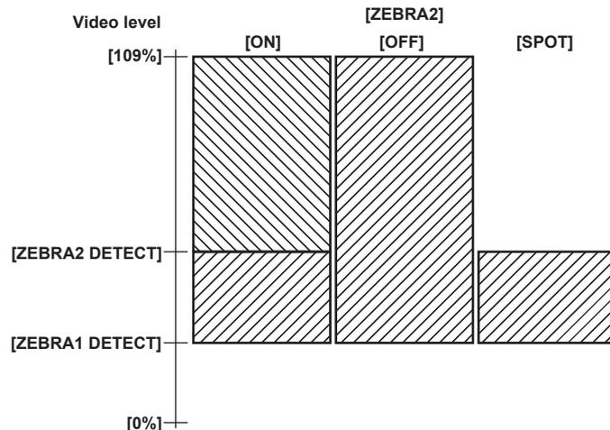
To display the zebra pattern in the video of the monitor output terminal (<SDI OUT2>, <VIDEO OUT>, <HDMI OUT>), set in the main menu → [I/F SETUP] → [OUTPUT SEL] → [MONITOR OUT ZEBRA].
