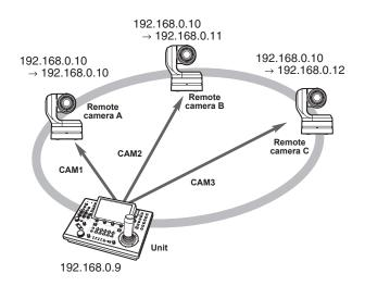
For the camera numbers for which "auto IP setting" is executed, the connection type becomes "LAN" and the camera numbers are excluded from the setting targets the next time "auto IP setting" is executed.
