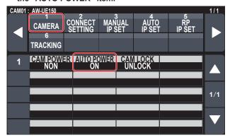
3. Turn the F2 dial to select "ON" and press the F2 dial. The power of remote cameras whose setting in the "CNNCT MD" item in the "CONNECT SETTING" SYSTEM menu is set to either "Serial" or "LAN" turns on when the unit's power is turned on.
