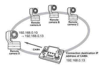
When you connect a remote camera for which the IP address has been changed using a personal computer or other device after a link was set to the unit with auto IP setting and then execute "RENEW", the same IP address as was set when auto IP setting was executed the first time is set again for the corresponding camera.
