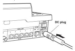
When the unit will not be used for a long time, turn off the power switch and remove the DC plug for the external DC power supply to save power.
