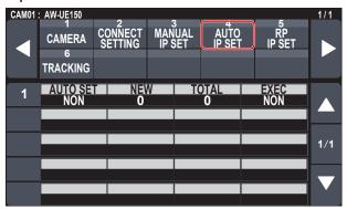
The number of devices currently being managed by the unit (All remote cameras and the newly detected number of devices are displayed in "NEW" and "TOTAL".)
