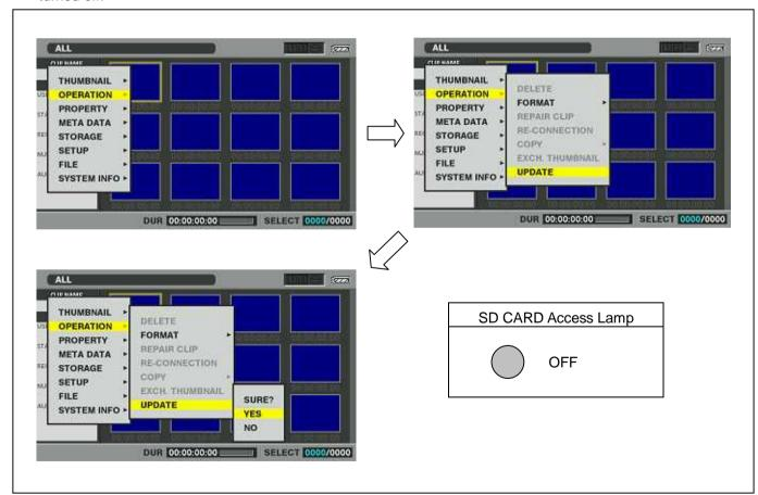
5. Update program is started and the message "PREPARING FOR UPDATE" appears on screen. In this timing, it is doing preparation such as the confirmation of the data of the updating. In this time, Access Lamp of SD CARD slot is turned on.
