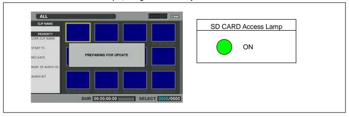
6. When shifting to the update process of the flash microcomputer, following screen is displayed. In this timing, it is doing preparation such as the confirmation of the data of the updating. In this time, Access Lamp of SD CARD slot is flash.
