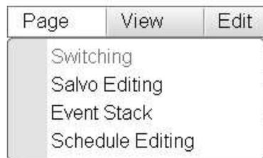
**View Menu** – The View menu opens to a listing of toggle functions that allow you to quickly open/close the flyout display windows or hide/unhide the switching level columns.
