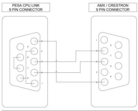
Note: If you have connections on the AMX/Crestron device that are not supported, then you must loop-back these connections on the PESA side. Example - Pins 4 & 6 or 7 & 8
