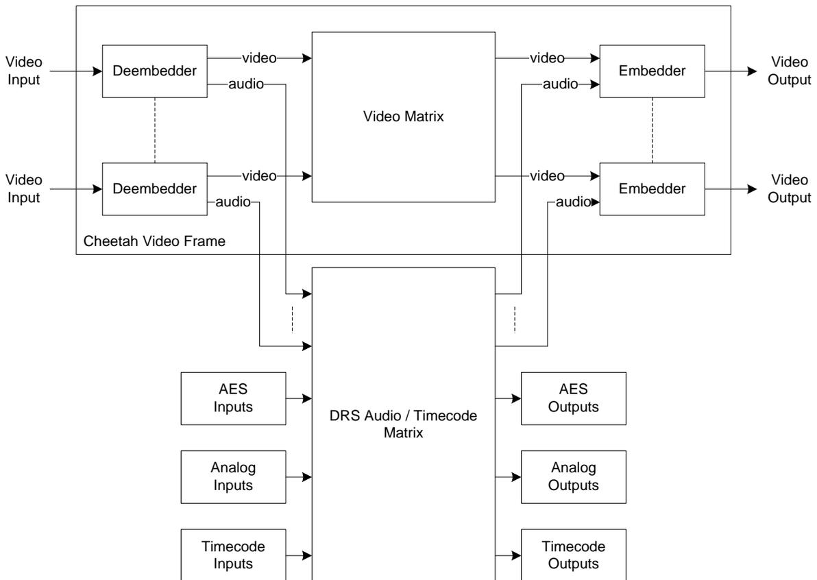
Figure 1 - Cheetah Video/Audio Routing System with Deembedders and Embedders Block Diagram
