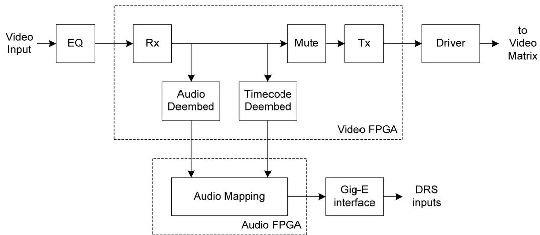
Figure 2 - Deembedder Card Single Channel Block Diagram
