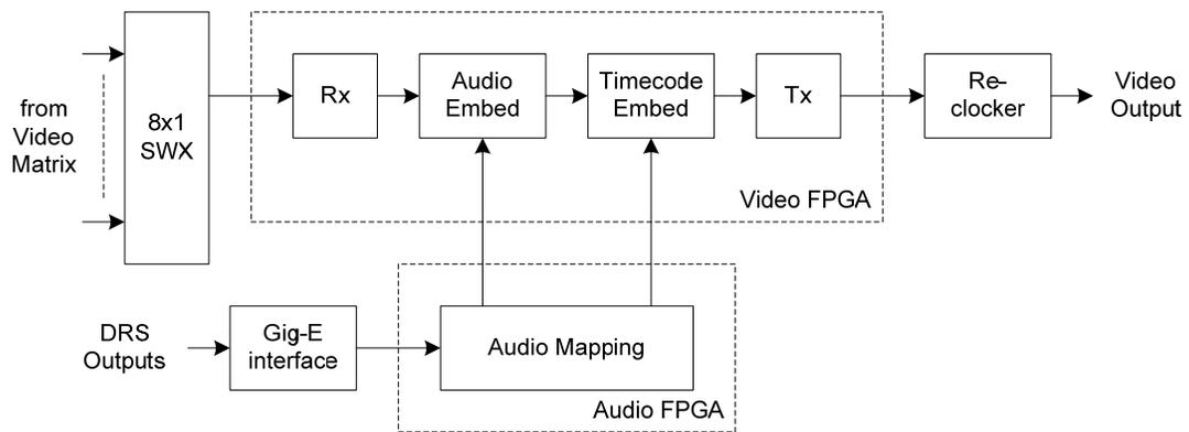
Figure 6 - Embedder Card Single Channel Block Diagram
