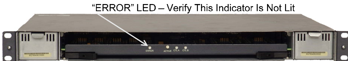
Figure 3-28 ERROR LED Location
