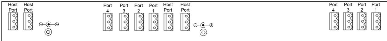
Figure 2. Dual 4x1 RCP Panel Port Expander Rear Panel
