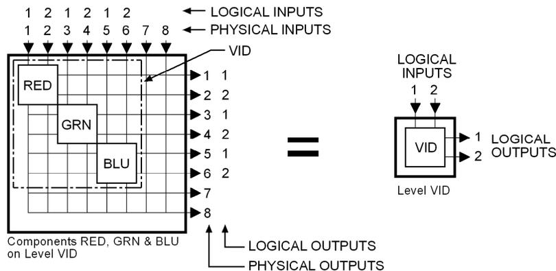
As a general rule, users control the switching of levels, but component switching is handled automatically by the switching system. In the example above, a user could specify a single logical switch, such as VID Input 1 to VID Output 2. This would result in Win3500Plus taking three physical switches by activating crosspoints (1,2), (3,4) and (5,6).
