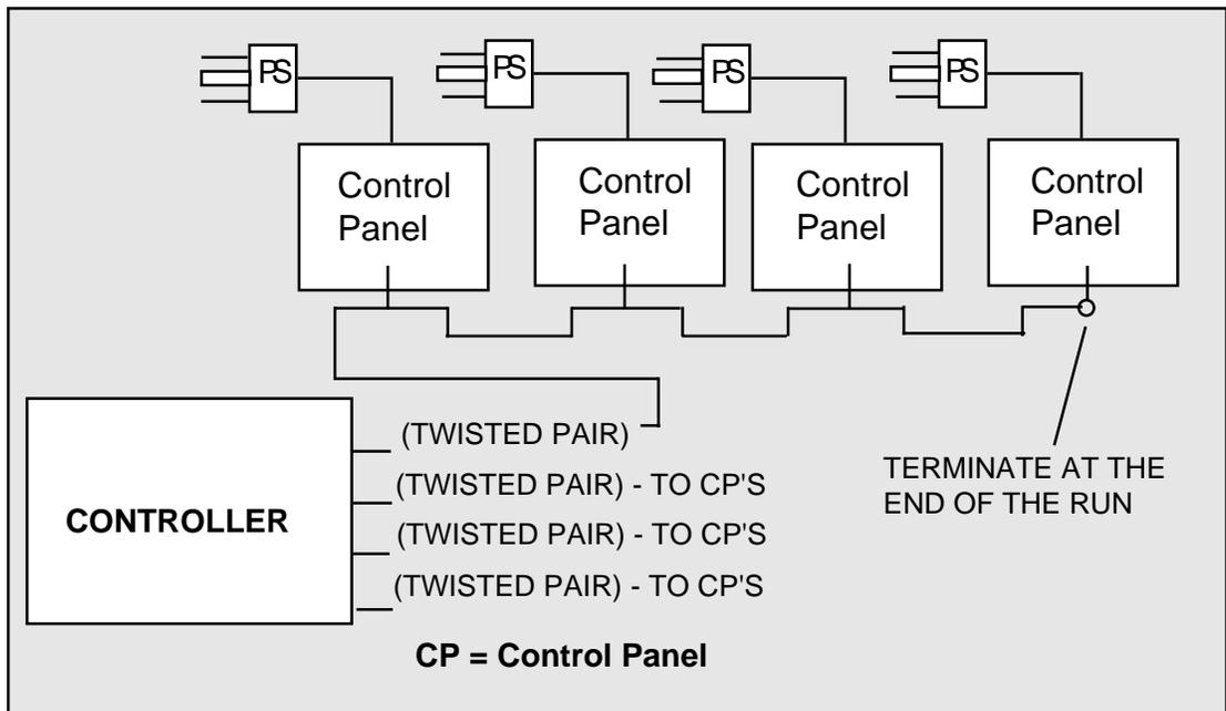
Figure 2-3 Typical Control Panel Controller Interconnection
