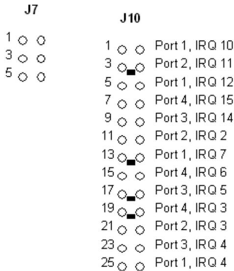
**Figure 12. Factory Settings, Interrupt Jumpers**
