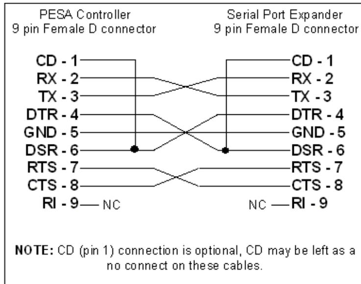
**Figure 4. RS-232 Cable Diagram**
