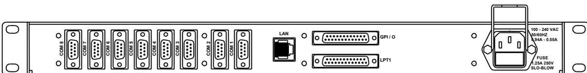
Figure 3. Serial Port Expander Rear View
