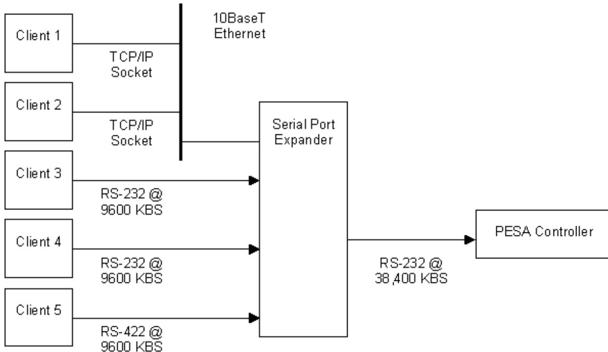
Figure 1. System Level Block Diagram, Single Output
