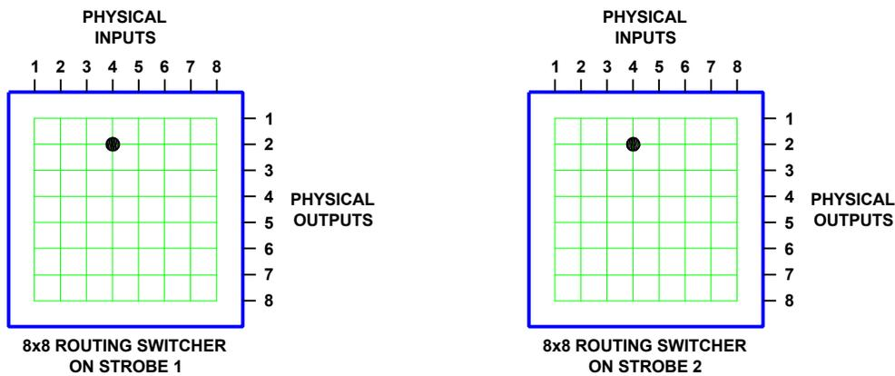
Figure 26. Matrix Space, Two Routing Switchers on Two Strobes
