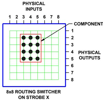
**Figure 27. Output Offset, Single Routing Switcher**
