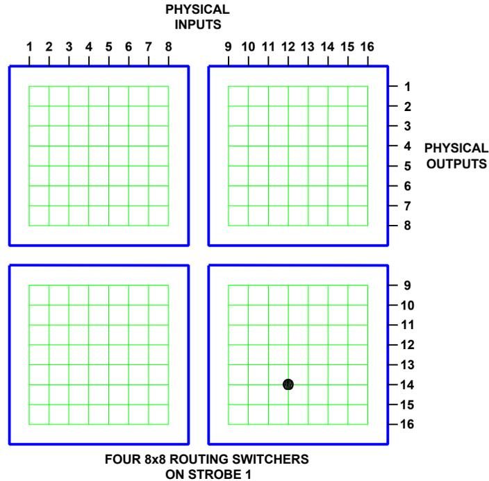
Figure 25. Matrix Space, Four Routing Switchers on One Strobe
