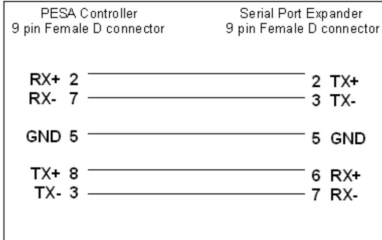
Figure 5. RS-422 Cable Diagram
