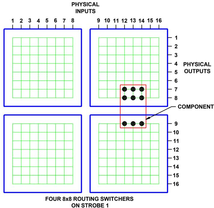
Figure 28. Output Offset, Multiple Routing Switchers
