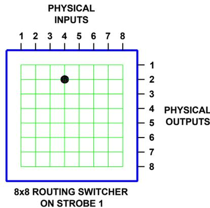
**Figure 24. Matrix Space, One Routing Switcher on One Strobe**
