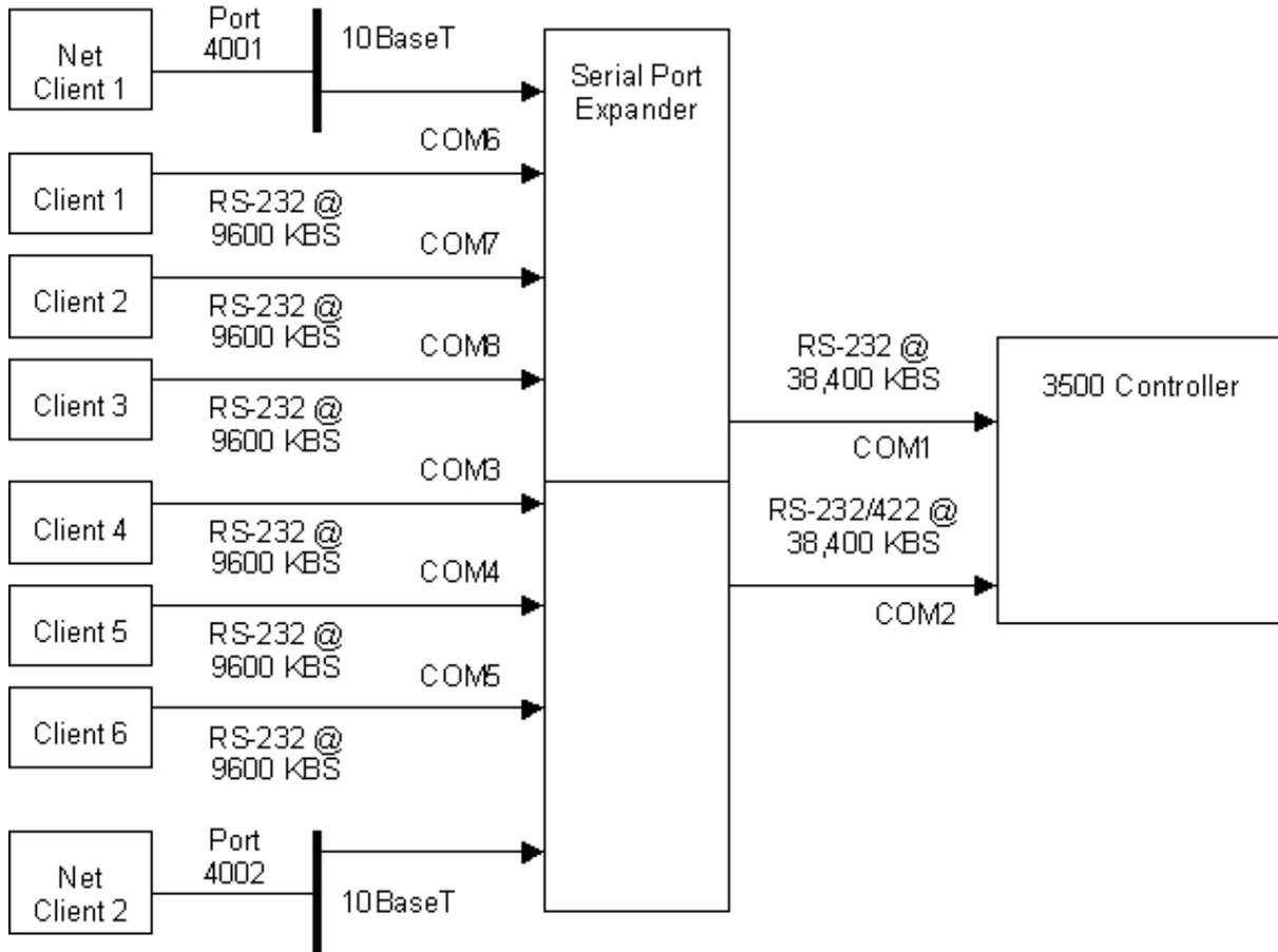
**Figure 15. System Level Block Diagram, Multiple Outputs**
