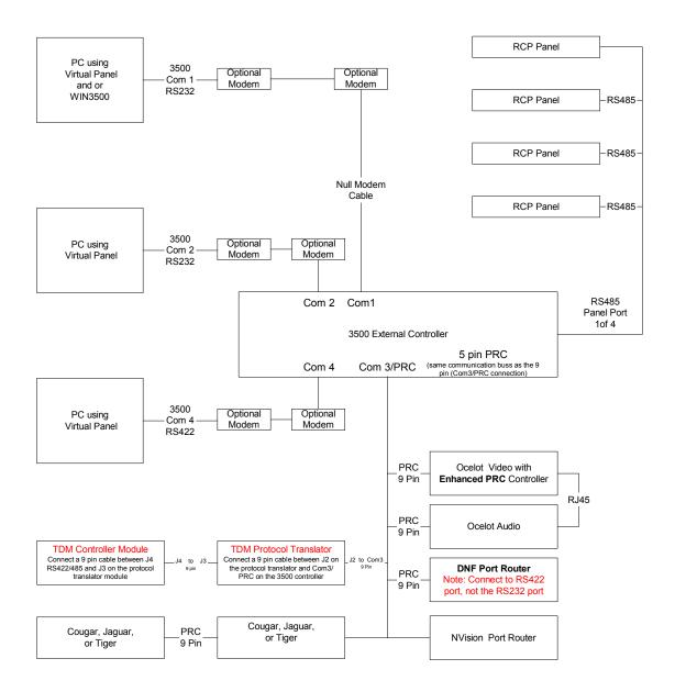
In this configuration, the 2 each Virtual Panels and the WIN3500/Virtual Panel can control the Cougar, Jaguar, Tiger frames and or the Bobcat, LNS-8, Ocleot frames simutaneously.
