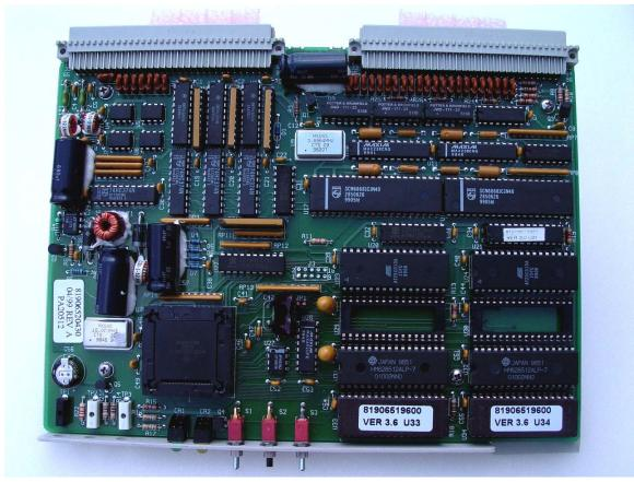
New style hardware using flash ram. May be upgraded to 3500 PRO/LE and 3500 PRO by user in the field
