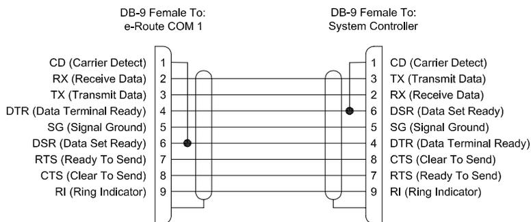
Figure 5. RS-232 CPU Link (Null Modem) Cable
