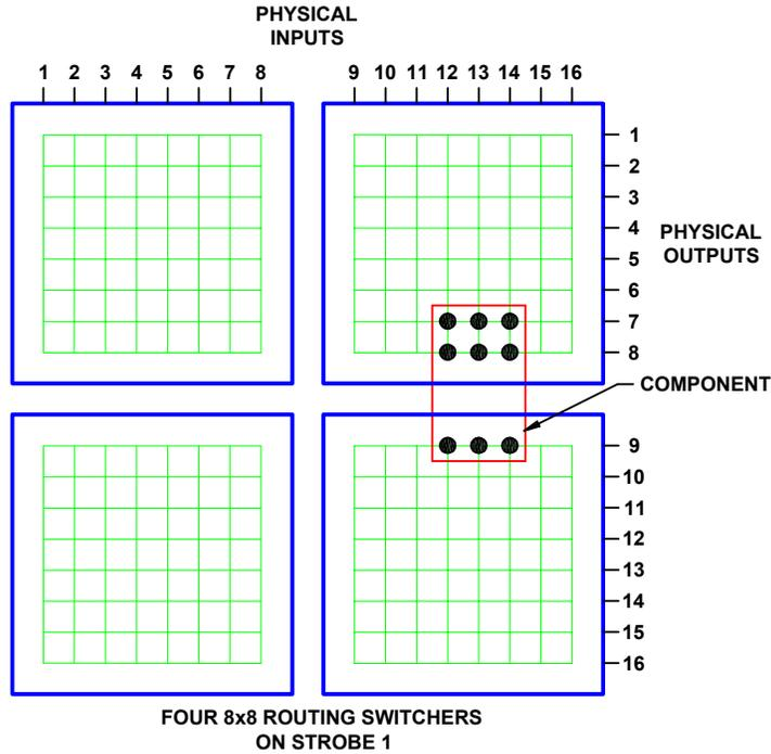
**Figure 54. Input Offset, Multiple Routing Switchers**
