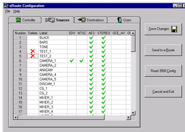
Figure 20. e-Route Configuration Sources Tab
