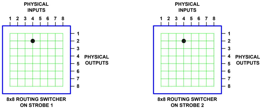
**Figure 59. Matrix Space, Two Routing Switchers on Two Strobes**
