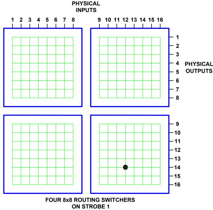
**Figure 58. Matrix Space, Four Routing Switchers on One Strobe**
