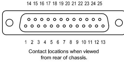
**Figure 7. GPIO Connector**
