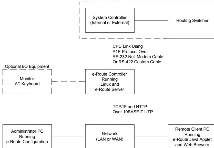
Figure 3. System Block Diagram
