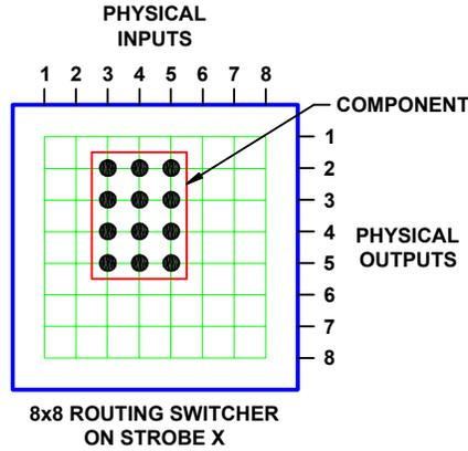
**Figure 53. Input Offset, Single Routing Switcher**
