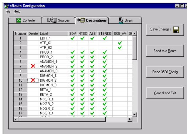
Figure 21. e-Route Configuration Destinations Tab
