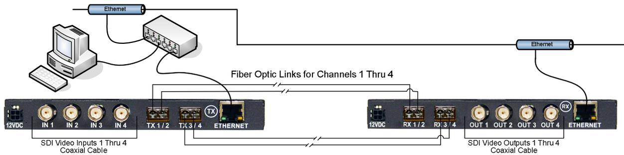
**Figure 2-4 Typical TX Direct to RX Installation**
