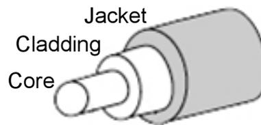
**Figure 3-1 Fiber Optic Cable, Basic Cross Section**
