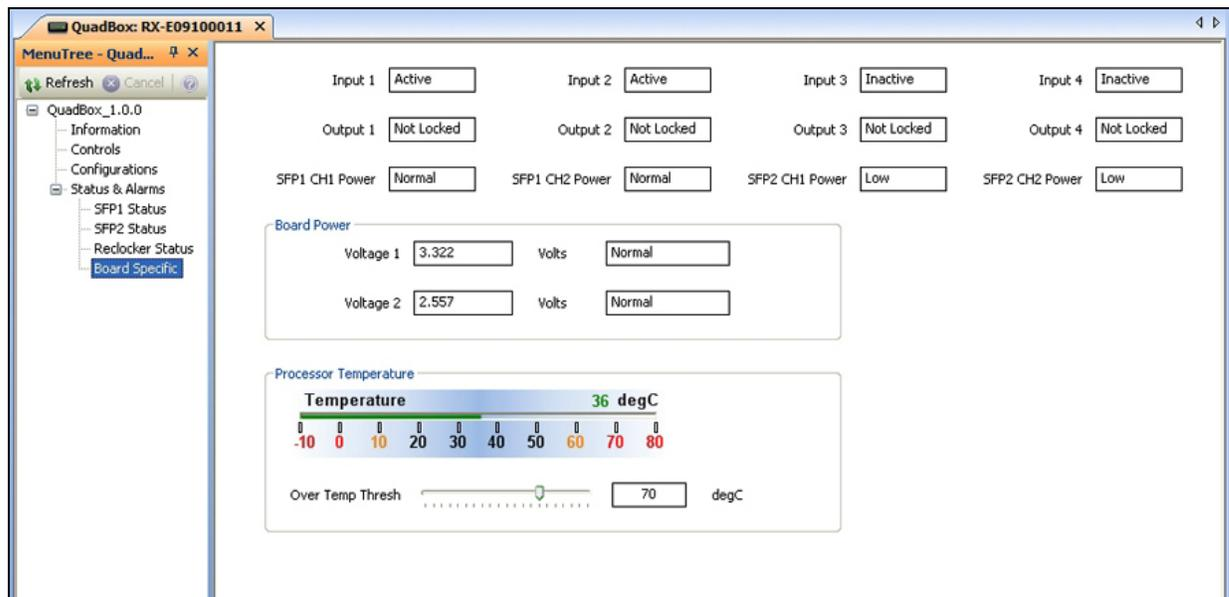
Figure 5-12 Example Board Specific Screen
