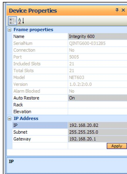
Figure 5-14 Changing IP Address from Device Properties Panel
