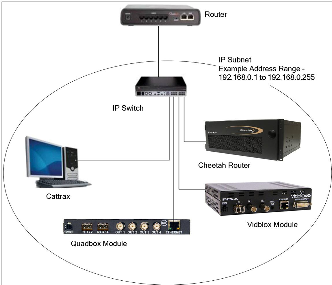
**Figure 5-13 Cattrax Installation Using an IP Switch to Connect Managed Devices**
