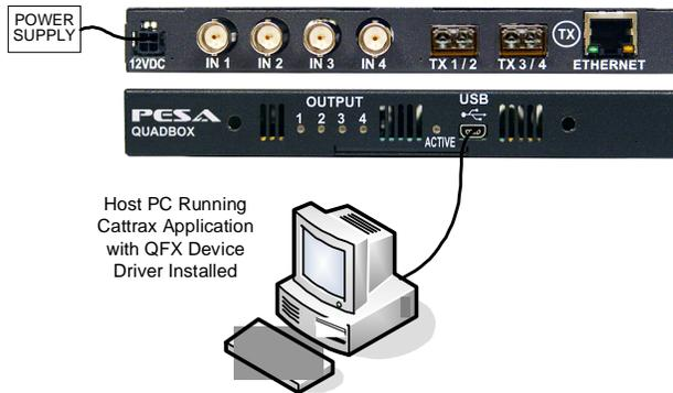
1. Apply power to the Quadbox module by connecting the external power supply to the module and to a source of primary power.
