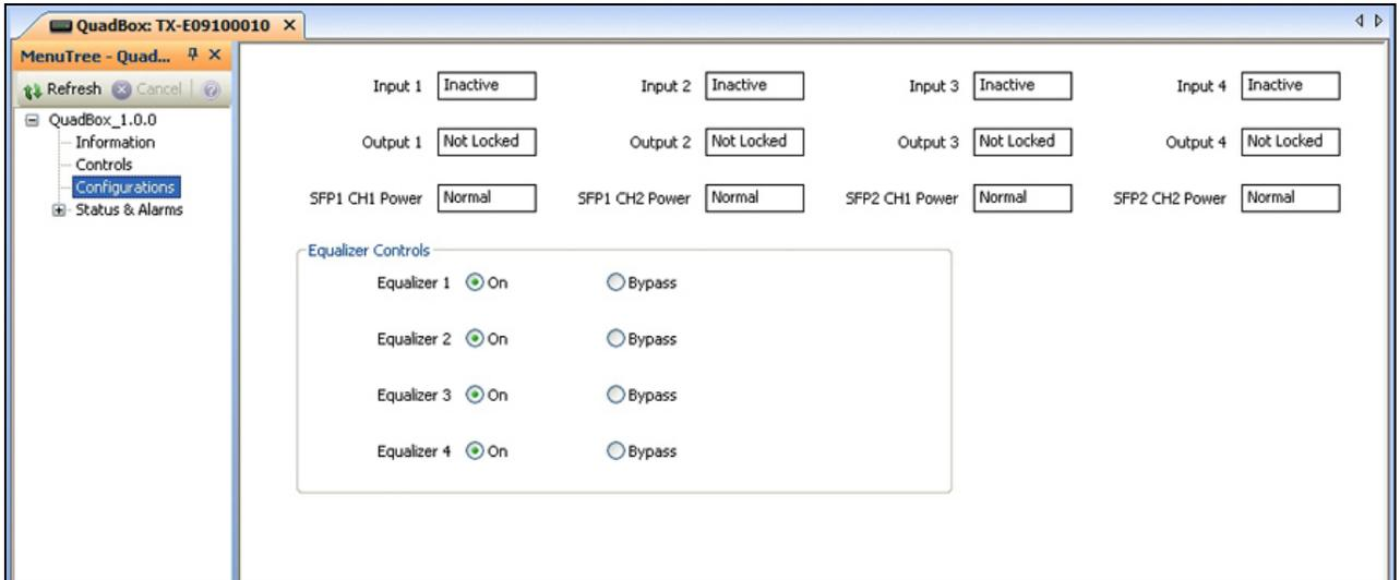
Figure 5-8 Example *Transmit* Module Configurations Screen
