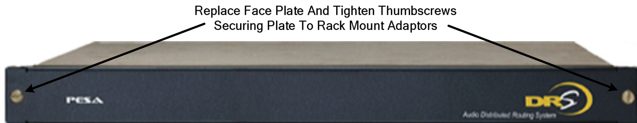
Figure 5-25 Front Panel Replacement
