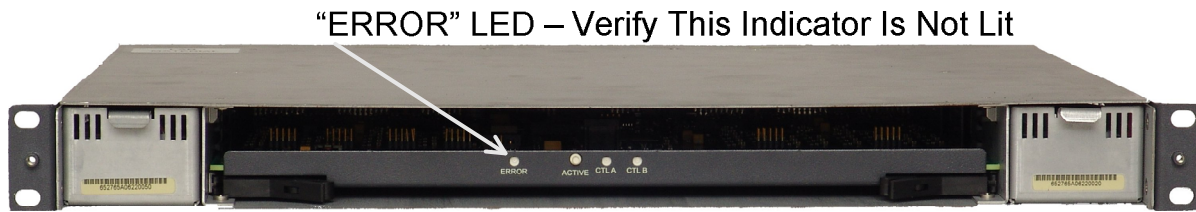
FIGURE 5-24 ERROR LED Location
