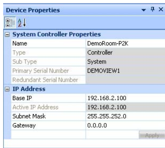
Figure 6-6 Example System Controller Device Properties Display
