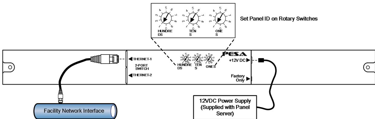
**Figure 4-14 RCP Panel Server Connections**
