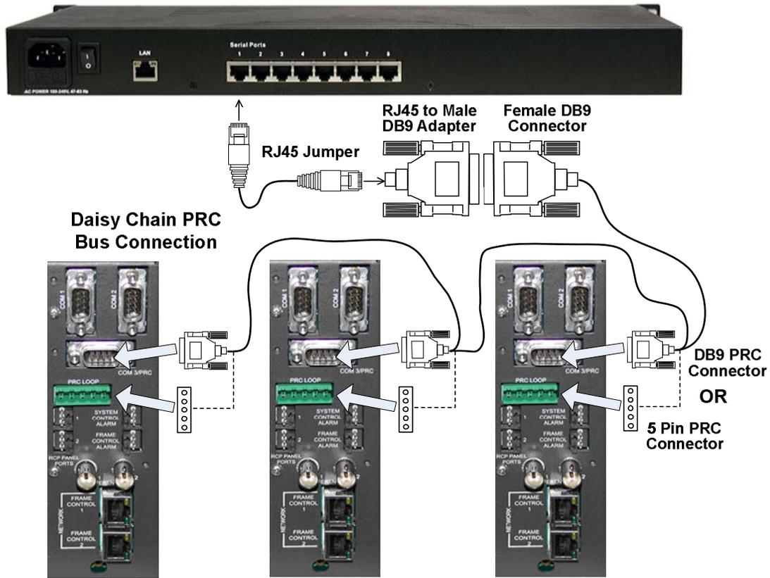
**Figure 4-7 Typical PRC Bus Installation**
