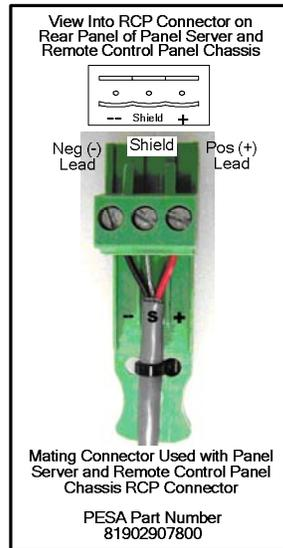
**Figure 4-16 Preferred RCP Connector Pin-Out Diagram**
