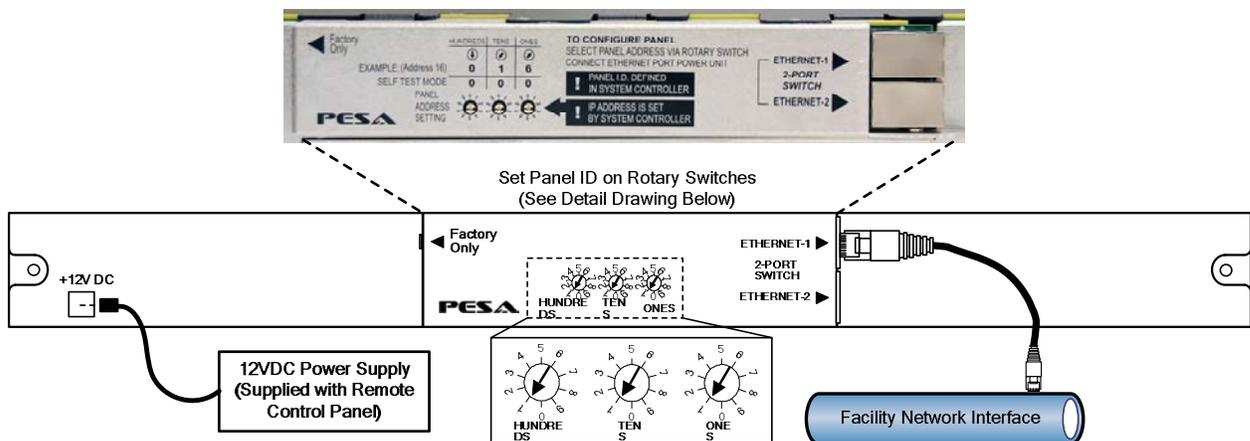
**Figure 4-12 Network-Based Remote Control Panel Connections**
