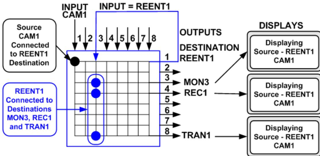
Figure 5-25 Crosspoint Connections for a Reentry Function
