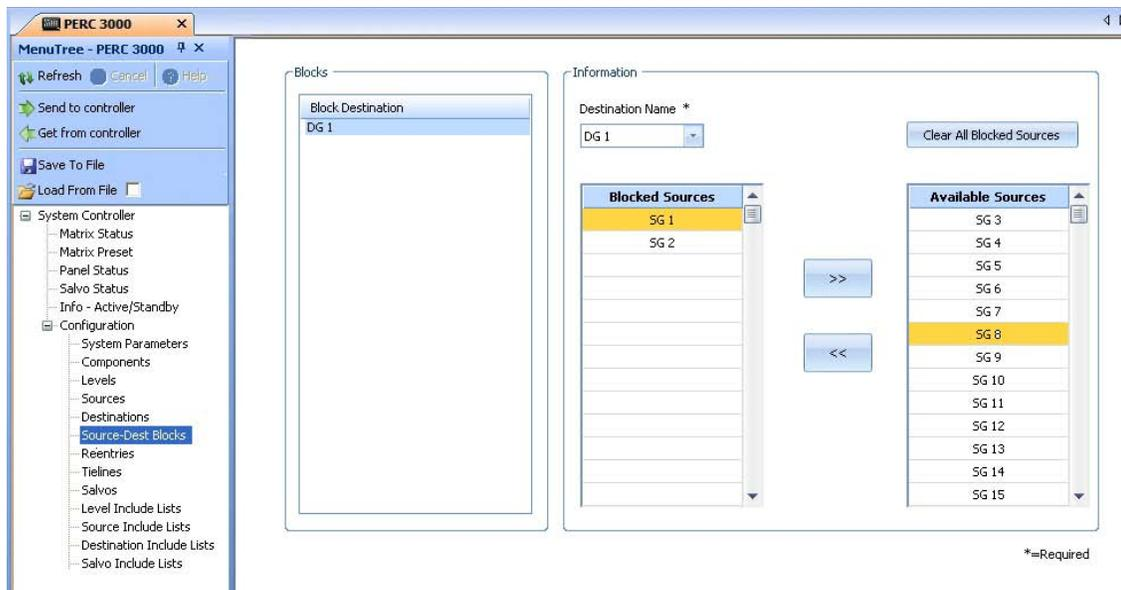
Figure 5-24 Source-Destination Block Configuration Page
