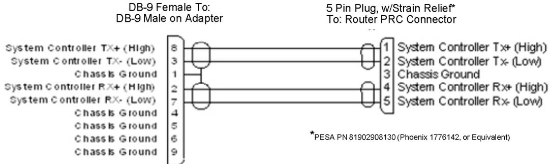
**Figure 4-10 RS-422 System Expansion Cable**
