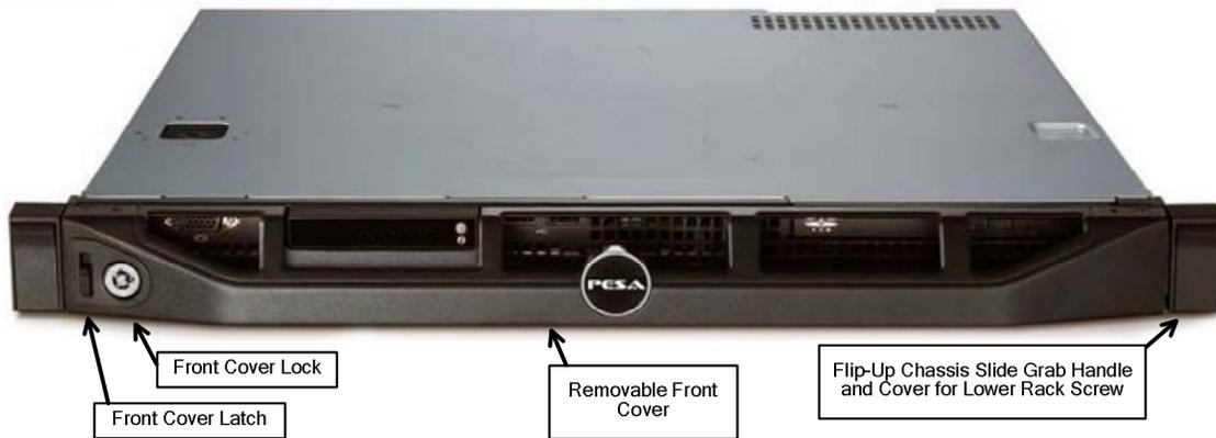
**Figure 4-1 PERC3000 System Controller - Front Cover in Place**
