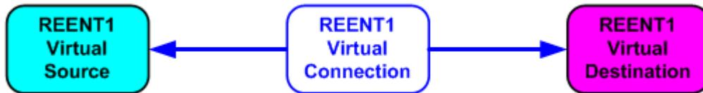
Figure 5-26 illustrates an example reentry path with the configuration name of REENT1. For this example, we illustrate a switching matrix with 8 physical inputs and 8 physical outputs. We have defined source names for all 8 inputs (with source ID numbers assigned for system tracking) and destination names for all 8 outputs (with destination ID numbers assigned for system tracking).
