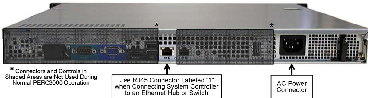
**Figure 4-2 PERC3000 System Controller – Rear View**
