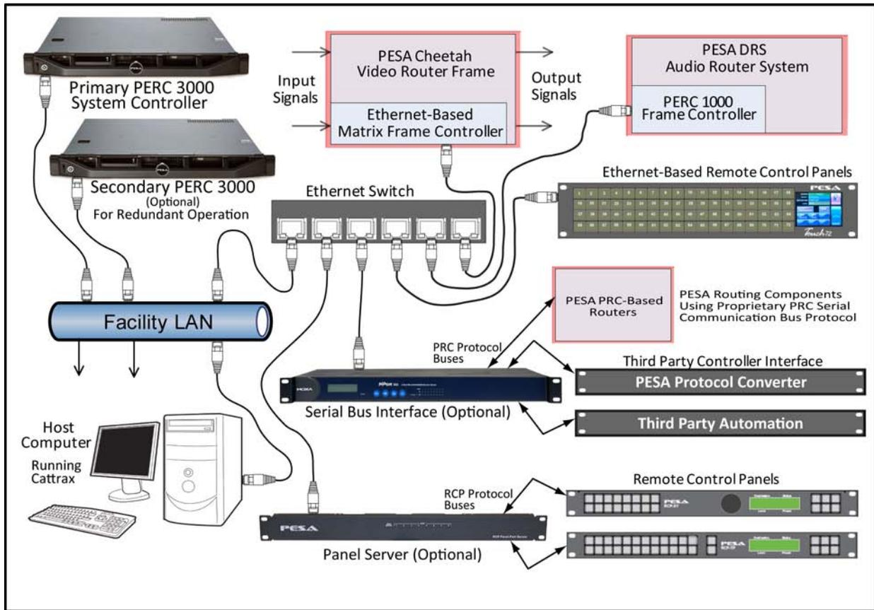
Figure 2-2 Typical PERC3000 System Controller Installation
