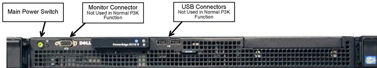
**Figure 4-3 PERC3000 System Controller - Front Cover Removed**
