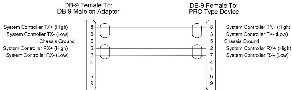
**Figure 4-8 RS-422 Serial Cable for PRC Bus**
