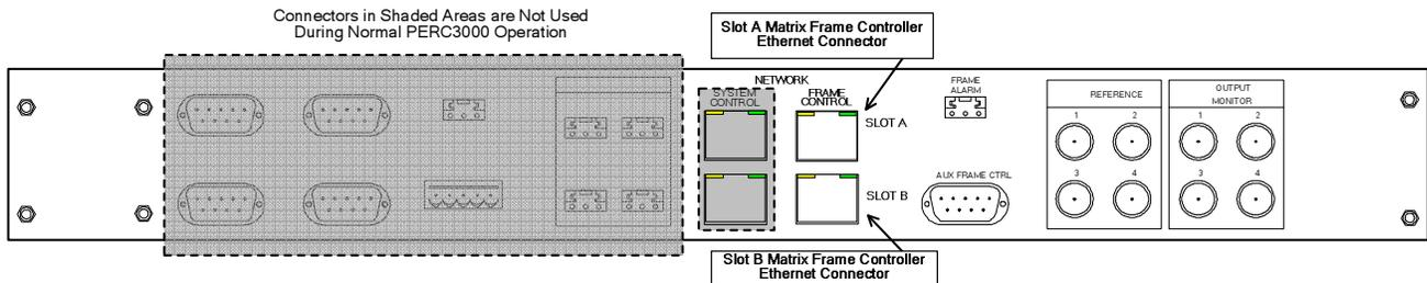
Figure 4-4 Typical Cheetah Video Frame Connector Panel
