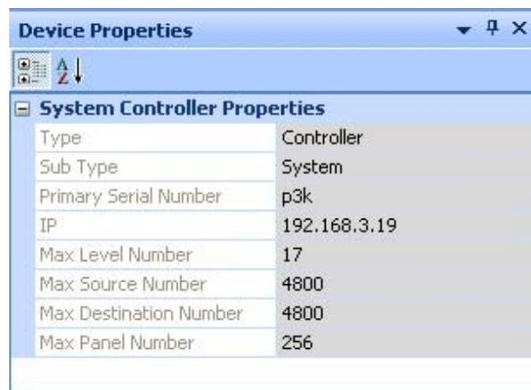
Figure 5-7 System Controller Device Properties
