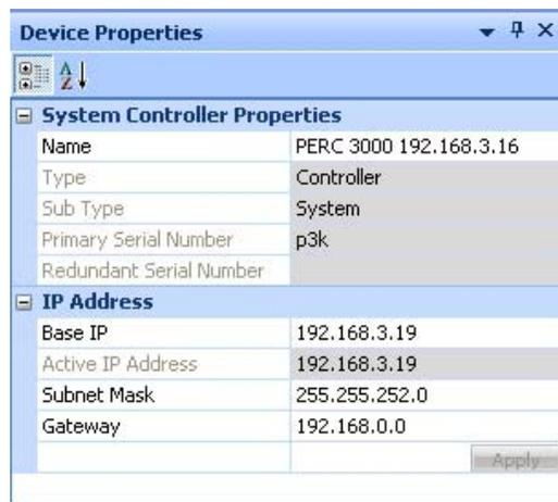
Figure 5-6 Example System Controller Device Properties Display
