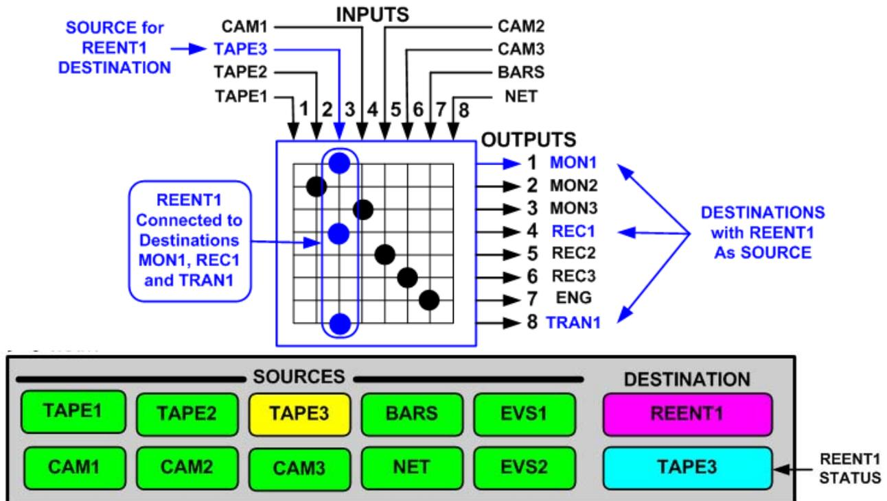
Figure 5-26 Crosspoint Connections for REENT1 Example and Panel Status
