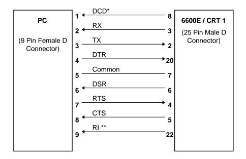
9 pin to 25 pin "Null Modem" Cable
