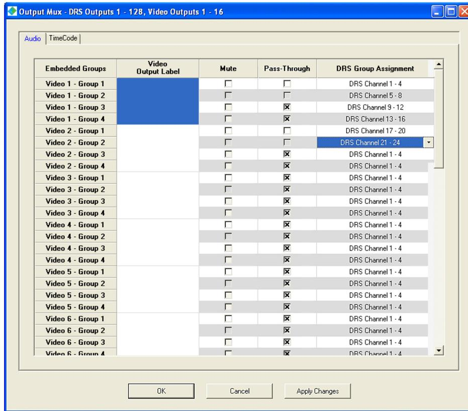
**Figure 5-13 Example Output MUX Setup Screen**
