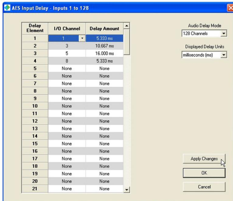
**Figure 5-23 Example Delay Setup Screen**
