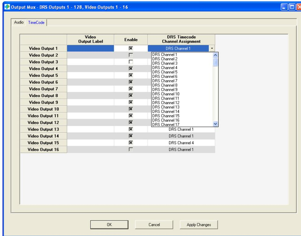
Figure 5-16 Mux Timecode Channel Assignment
