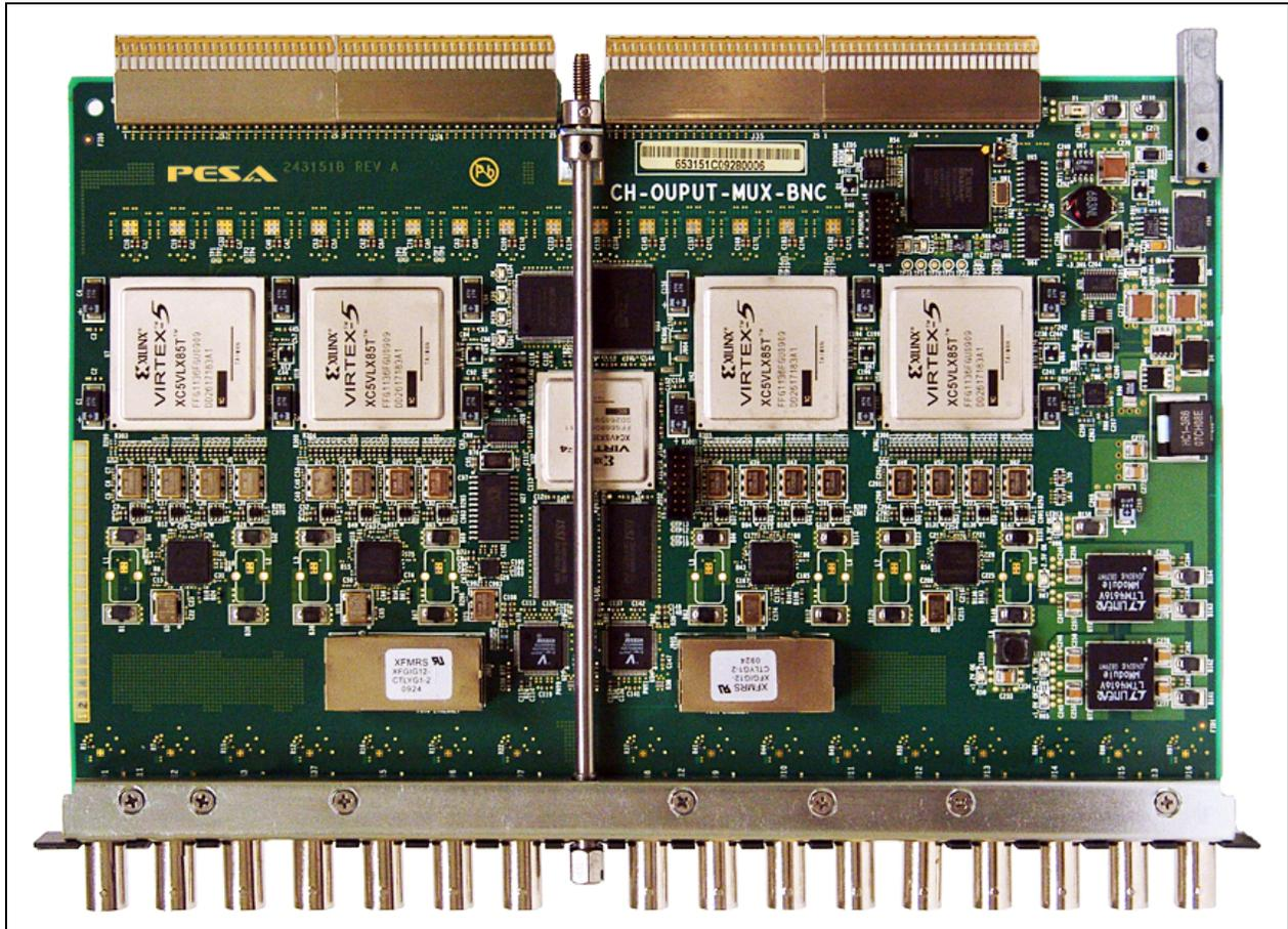
**Figure 2-3 Cheetah Output MUX 3G Video Card**
