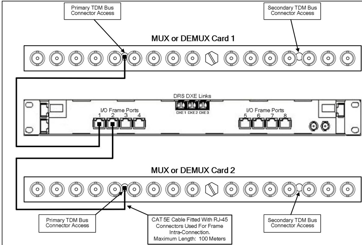
**Figure 3-5 Packet Audio Stream Connection
