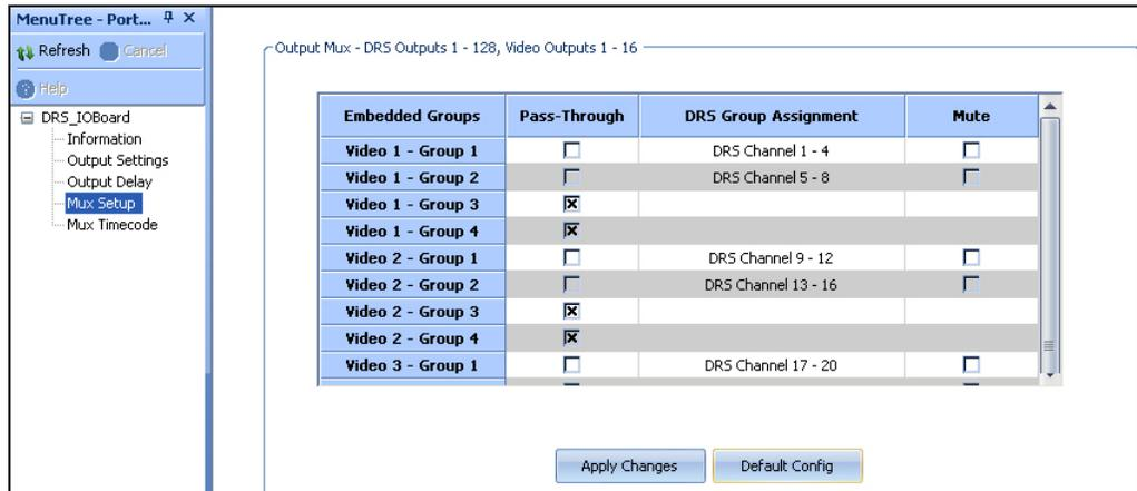
**Figure 4-11 Mux Setup Menu**
