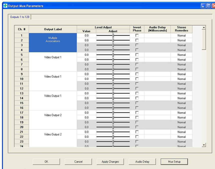
Figure 5-12 Example Output MUX Parameters Screen
