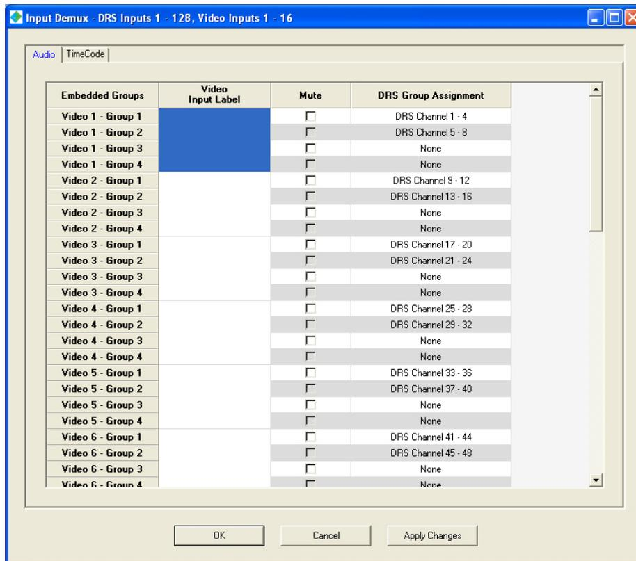
Figure 5-8 Example Input DEMUX Setup Screen
