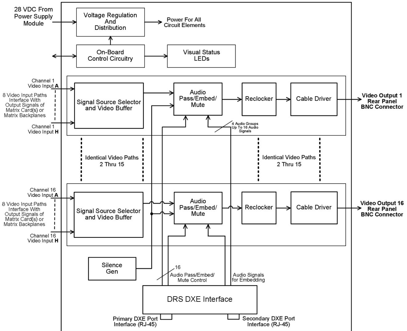
**Figure 2-4 Block Diagram – Output MUX Card**
