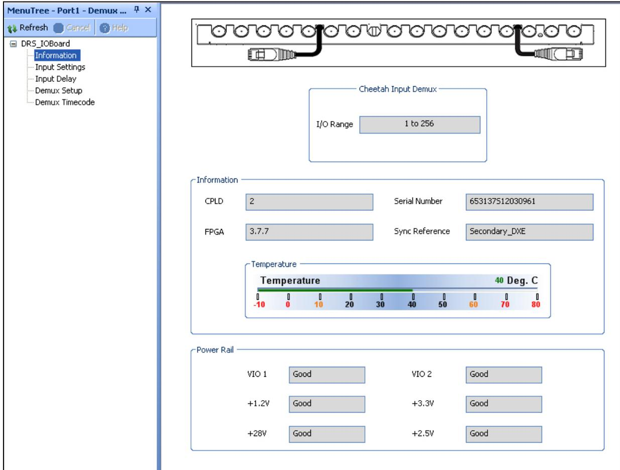
Figure 4-4 Typical MUX or DEMUX Card Information Display
