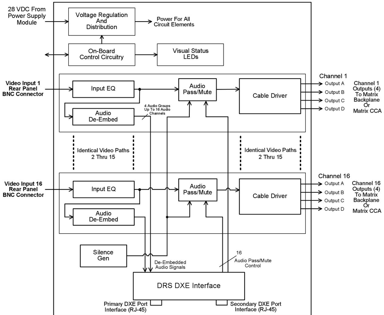
**Figure 2-2 Block Diagram – Input DEMUX Card**
