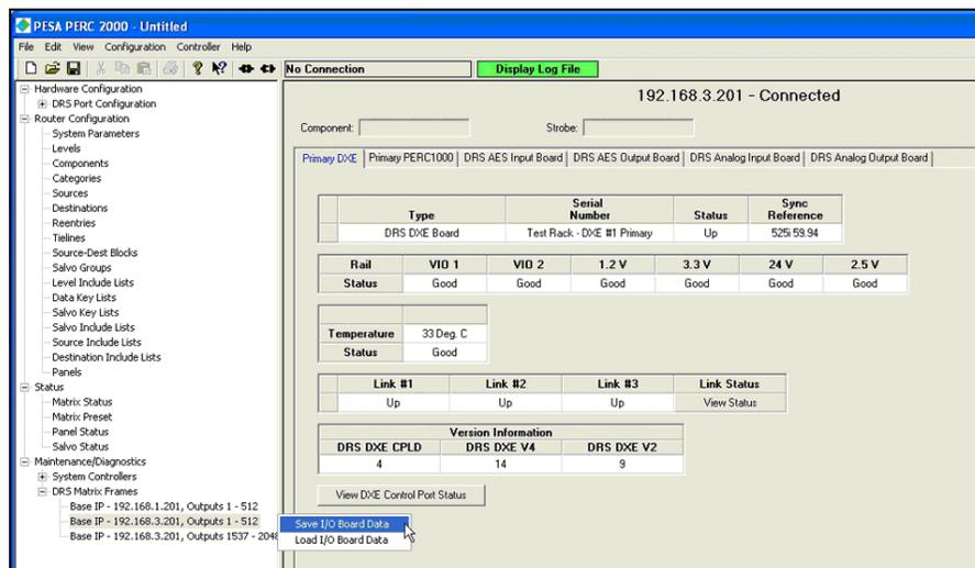
Figure 5-27 Audio Data Save and Load Commands
