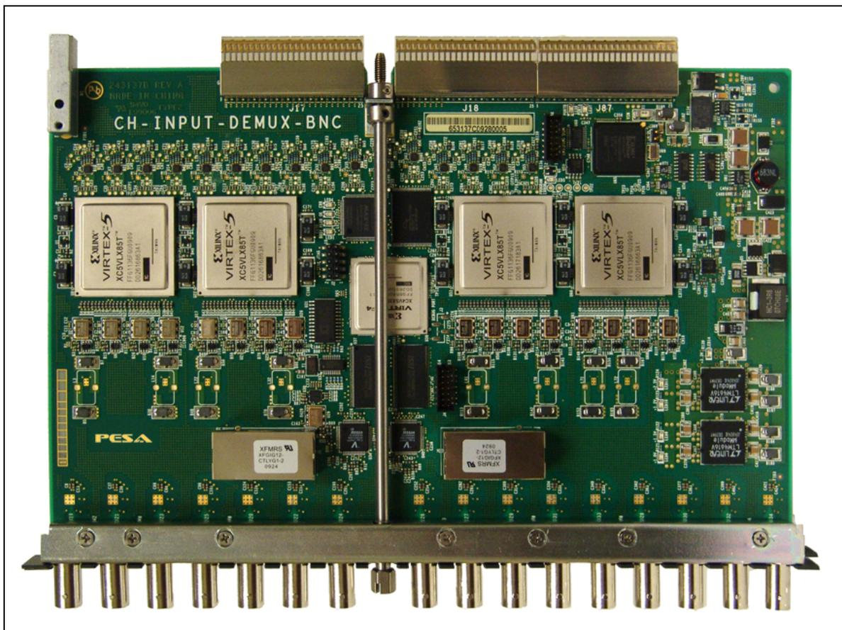
**Figure 2-1 Cheetah Input DEMUX 3G Video Card**
