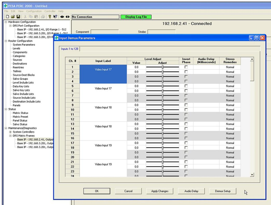
Figure 5-7 Example Input DEMUX Parameters Screen
