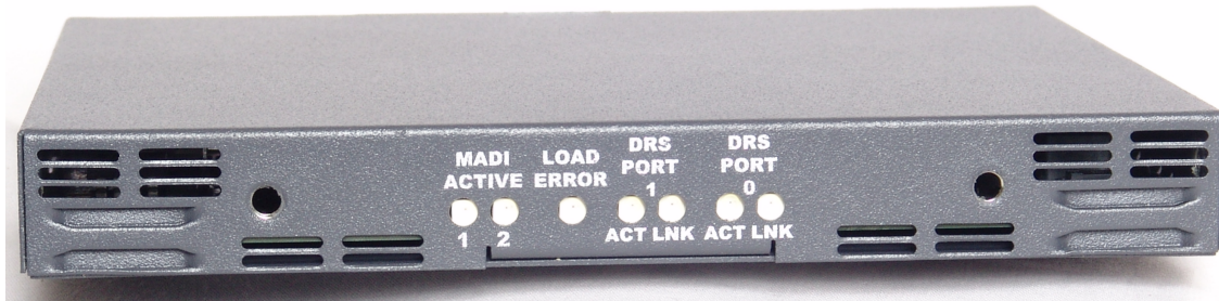
Figure 4-2 MADI Module Front Panel
