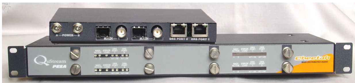
Figure 2-1 Cheetah DRS MADI Adapter – Typical Module and Rack Unit
