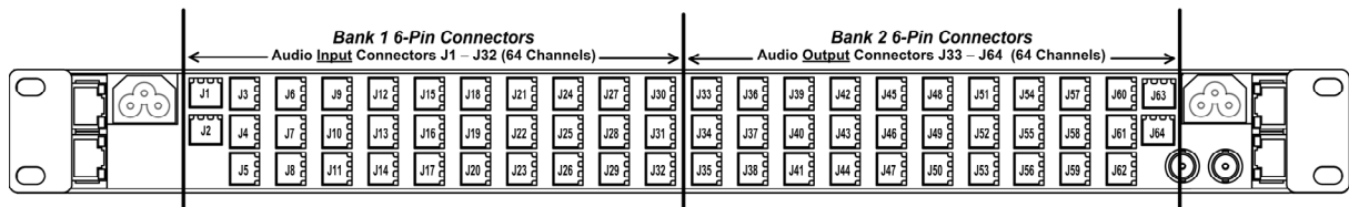
Figure 3-8 6-Pin Connector Rear Panel – Connector Numbering Layout
