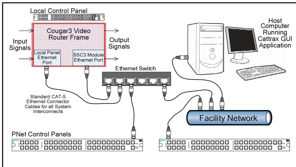
**Figure 2-7 Typical Cougar3 Network Installation**
