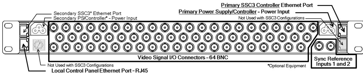
Figure 2-3 Rear Panel Connections – Cougar3 Stand-Alone SSC3 Configuration
