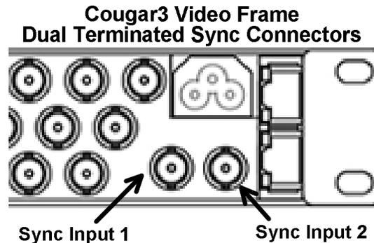
**Figure 3-6 Sync Reference Inputs**
