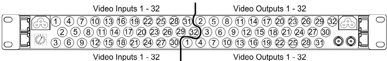
**Figure 3-5 Cougar3 Video I/O Connector and Channel Identification**
