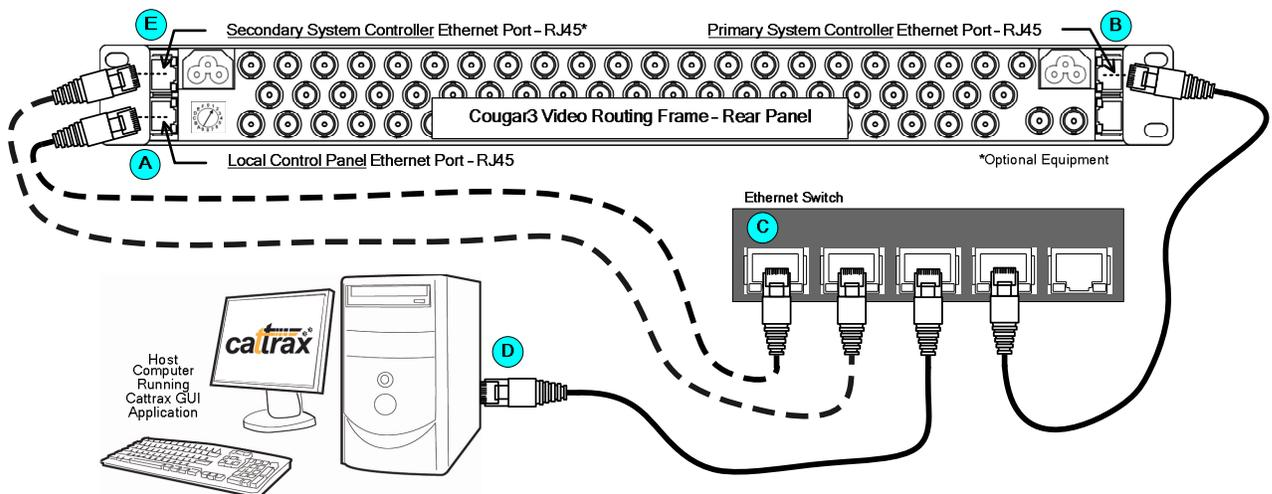
**Figure 3-3 System Cabling – Closed Ethernet Loop**
