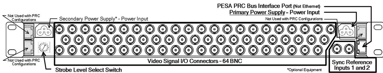
Figure 2-2 Rear Panel Connections – PRC Bus Installation
