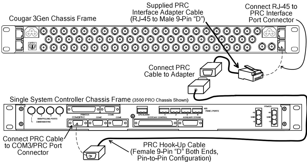
**Figure 3-2 Control System Connection**
