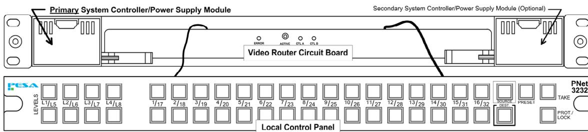
**Figure 2-1 Frame Component Layout (Typical)**
