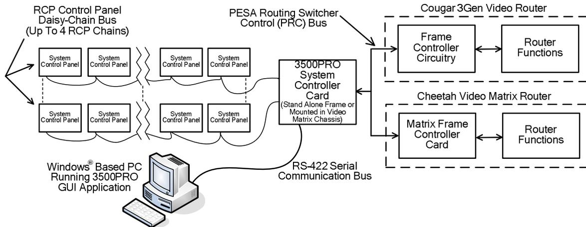
**Figure 2-4 Typical Installation – 3500PRO Controller**
