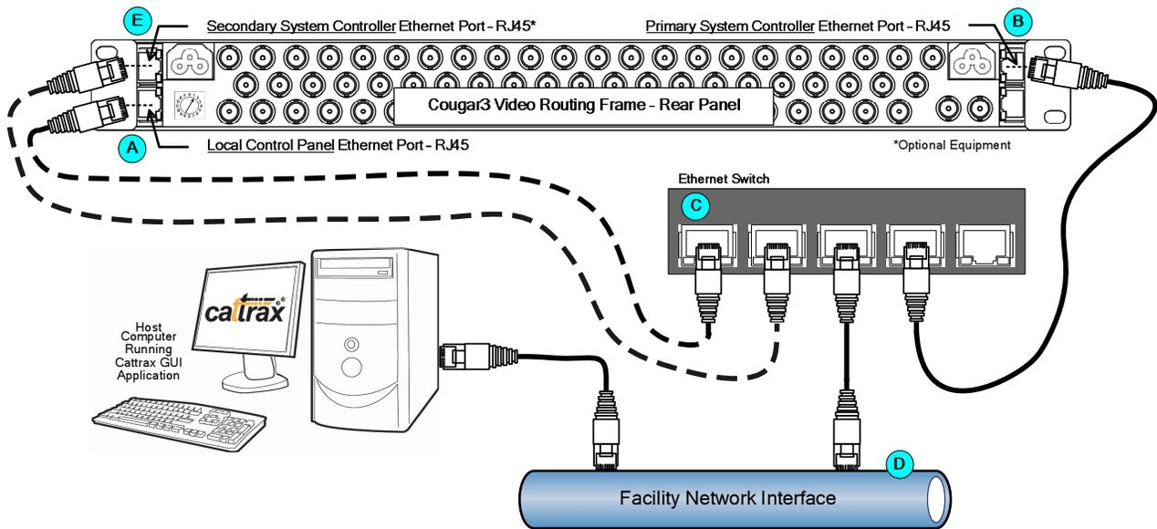
**Figure 3-4 System Cabling – Network Based Cougar3**
