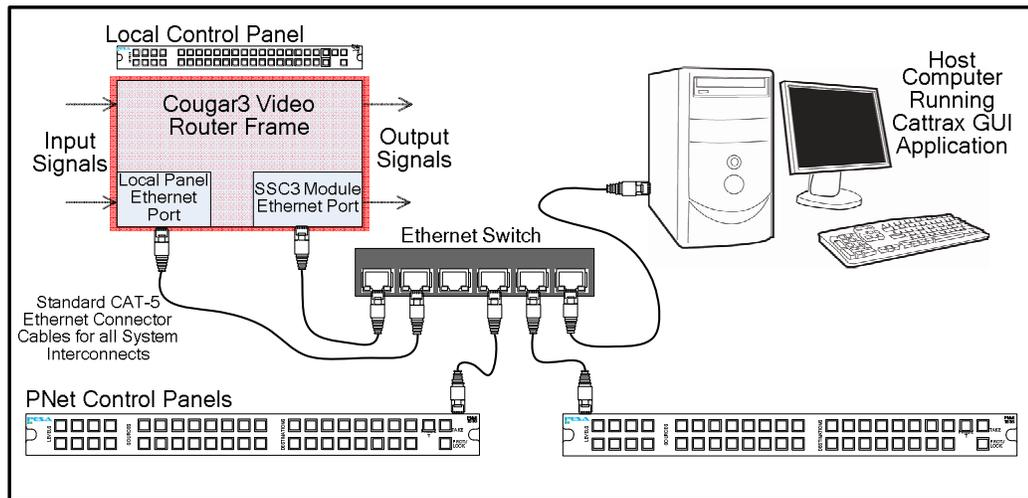
**Figure 2-6 - Typical Cougar3 Closed Loop Installation**
