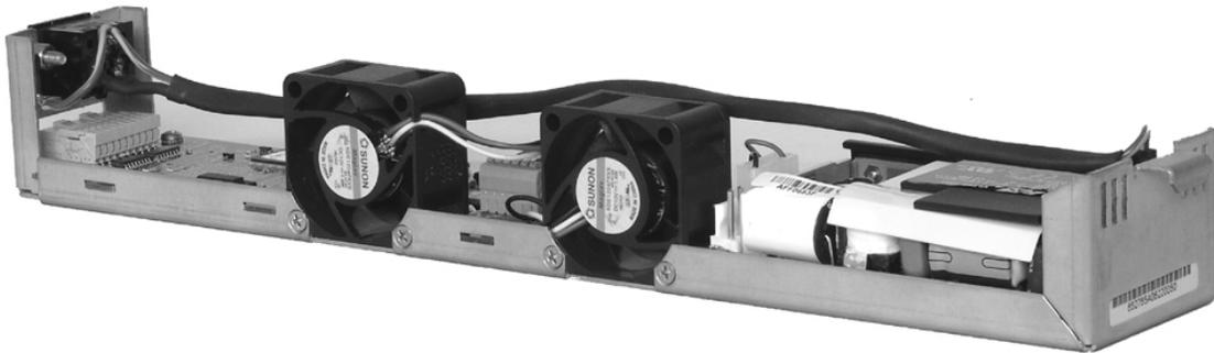
**Figure 2-8 Power Supply/Controller Module (Typical)**
