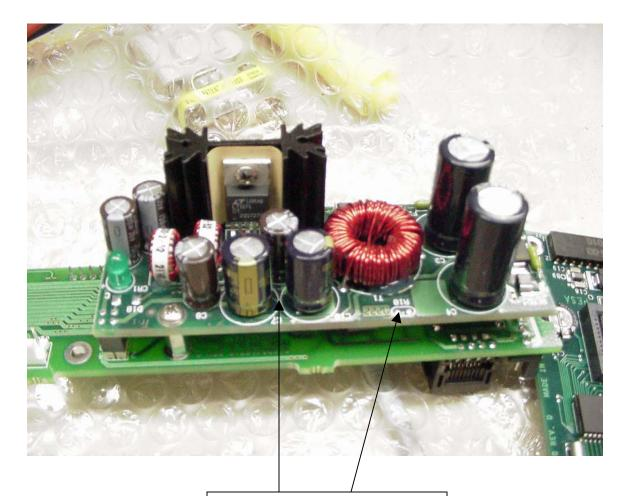
The Ocelot Audio Regulator – 81906519220 will not have a thermistor installed in the R10 position whereas the video regulator does. Other noticeable differences are in the capacitor sizes. (C7 & C18)
