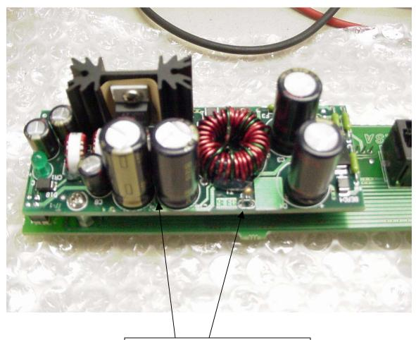
The Ocelot Video Regulator – 81906519170 has a thermistor installed in the R10 position whereas the audio regulator does not. Other noticeable differences are in the capacitor sizes. (C7 & C18)
