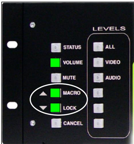
**FIGURE 102: Volume Up and Down Adjustment Control Buttons**
