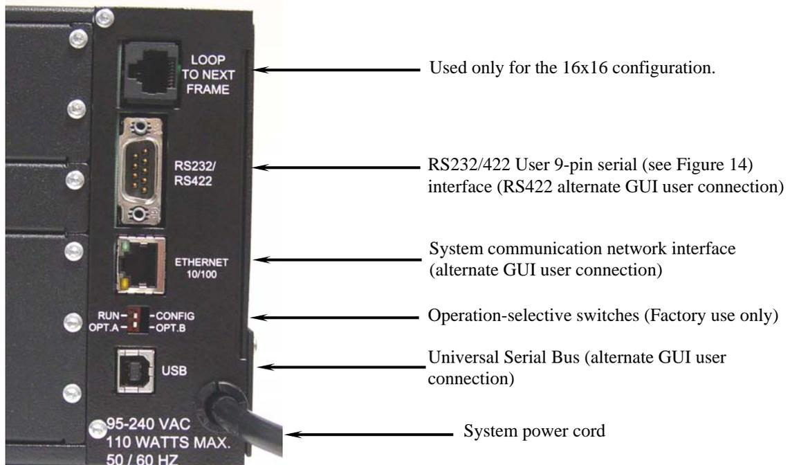
**FIGURE 13: System and User Connections**
