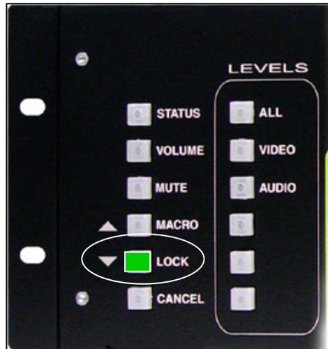
**FIGURE 24: The LOCK Key Location**
