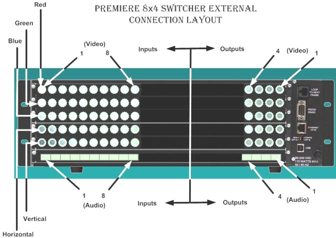
**FIGURE 15: Premiere 8x4 Connector Layout (Rear View)**
