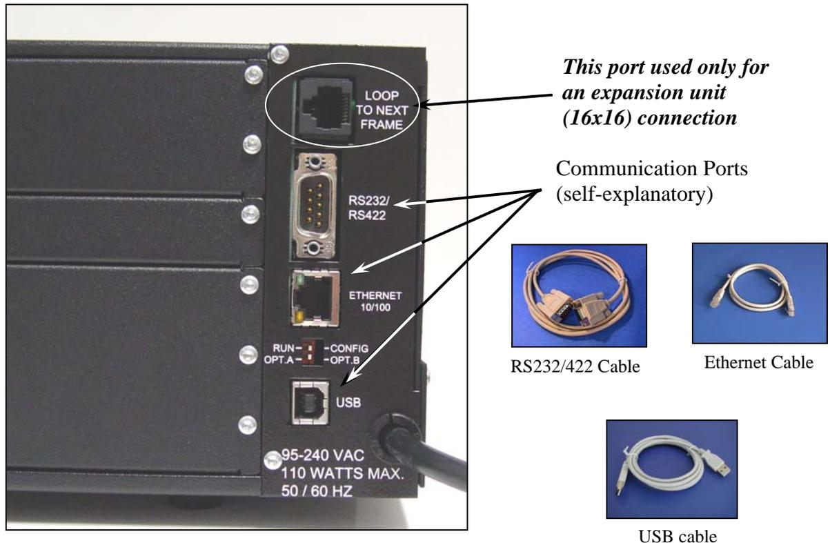
**FIGURE 30: An Individual Switcher's Connections**
