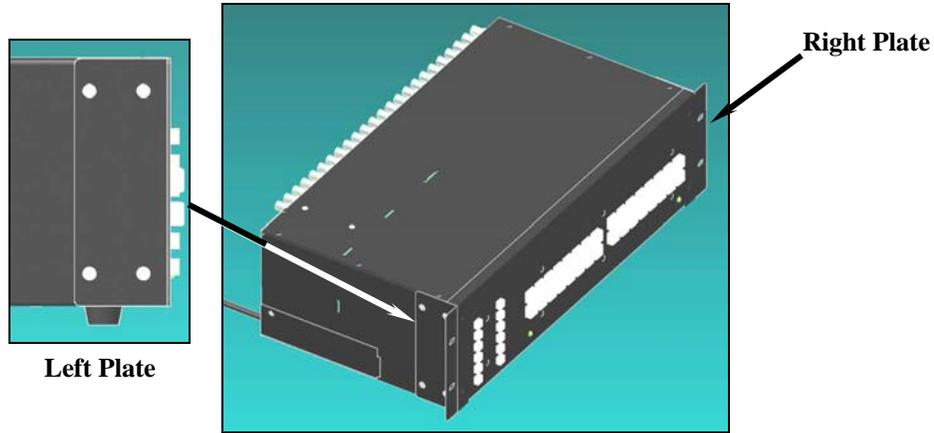
**FIGURE 4: 19-inch Rack Mounting Plate**
