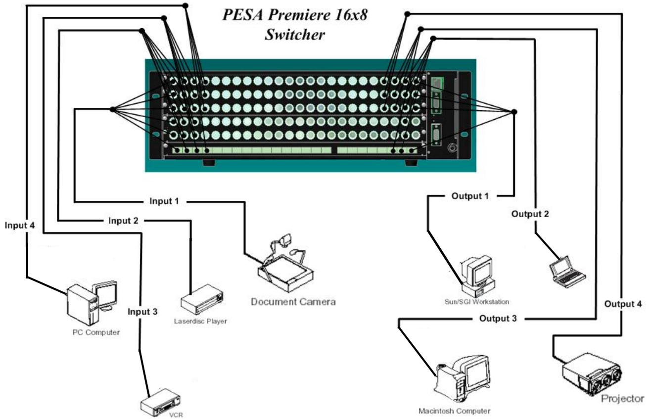
(Maximum peripheral capability for this system is 16 Input devices and 8 output devices)
