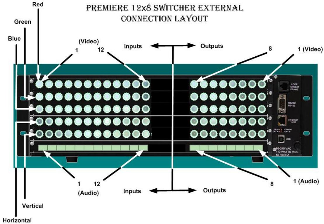
FIGURE 16: Premiere 12x8 Connector Layout (Rear View)
