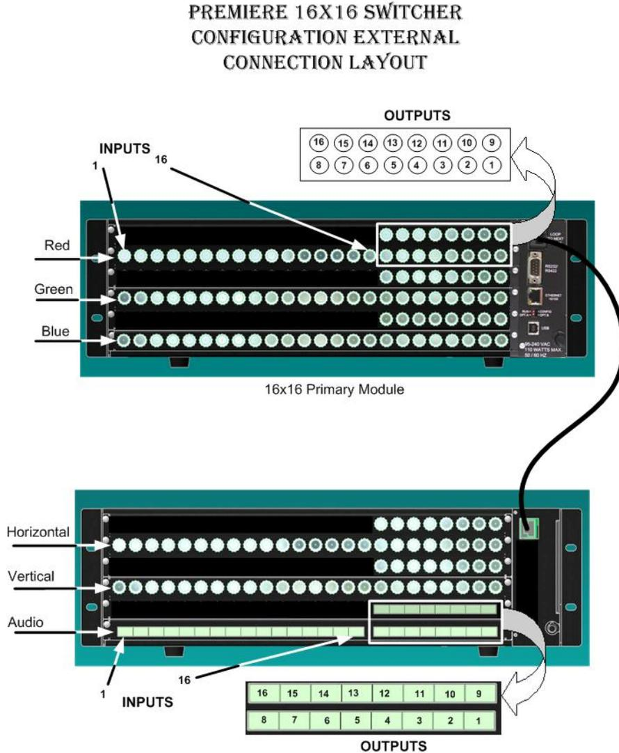
**FIGURE 18: Premiere 16x16 Connector Layout (Rear View)**
