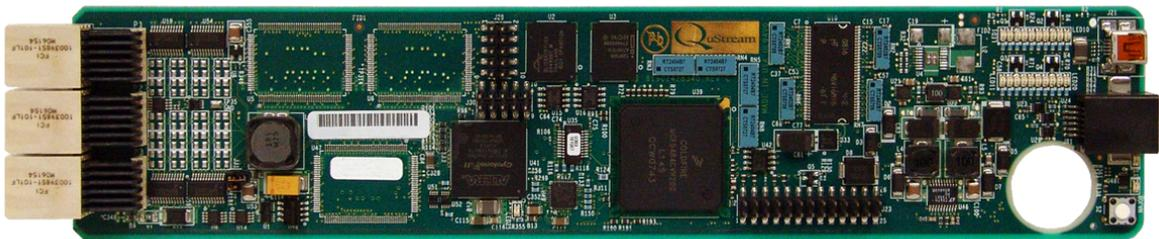
**Figure 2-1 NET603 Frame Controller Module**
