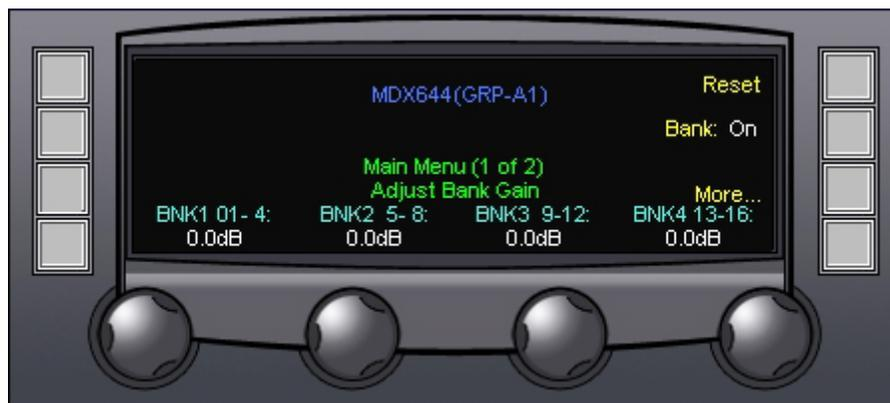
**Figure 4-2 Main Menu Screen Showing Linked Audio Channels**
