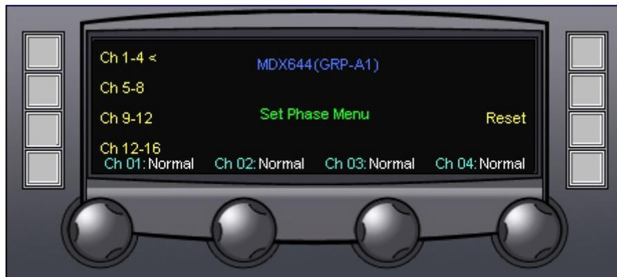
**Figure 4-13 Audio Output Phase Menu Screen**
