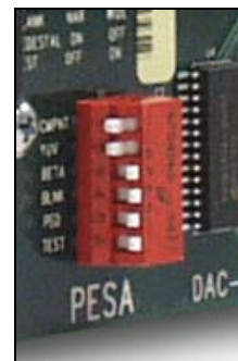
FIGURE 60: VDAC3101 Card Dipswitch Location
