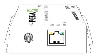
+5V DC: Connect to a 5V DC latch-locking power supply unit.
