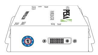
**SIGNAL LEVEL**: Adjust the 8-level signal equalization control to the received DVI signals. The DVI signal level varies from 0 (strongest) to 7 (weakest) for respective transmission length from longest possible range to short distance. Adjust the signal level may cause overpowering issue that would shorten the product life significantly!
