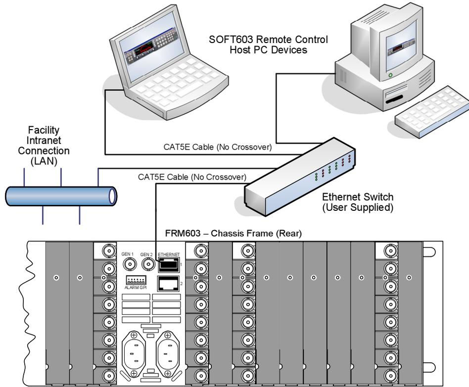
**Figure 3-2 Connecting Multiple Host PCs to a Local Area Network**
