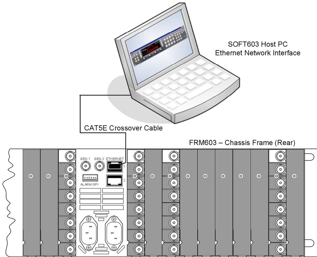
**Figure 3-1 Direct Connection of Host PC to Integrity Frame**
