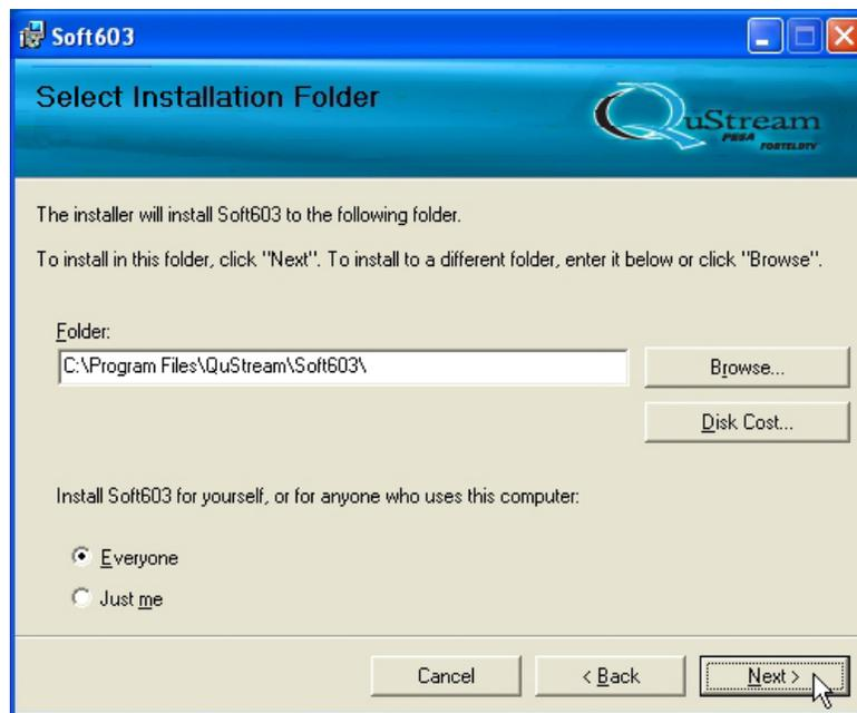
There is an additional button on the install folder prompt labeled **Disk Cost**. Clicking this button opens a display screen indicating the capacity and free space of hard disk drives in the PC, and the memory requirements of the SOFT603 application. An example of this screen is shown below. Click **OK** to exit this screen.
