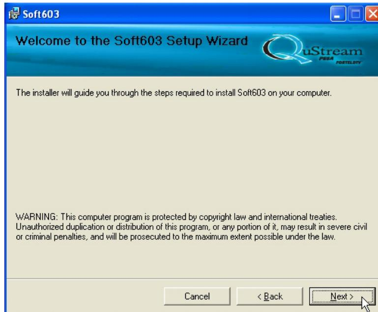
5. By default the auto-install function creates the folders shown below for the SOFT603 application. If you wish to install the software in a directory or folder other than the default, click **Browse** and navigate to the destination. At the bottom of the prompt screen you are given the option of installing the software to be available to everyone who uses the PC, or only to the user performing the installation. Click **Next** to begin installation.
