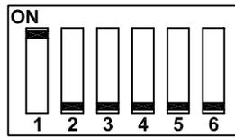
Figure 12. Front Panel DIP Switch
