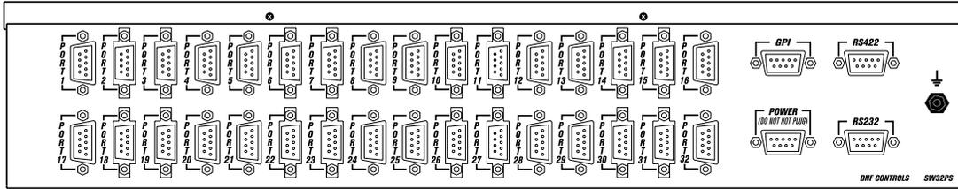
Figure 1. RS-422 Port Switcher Rear View
