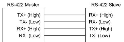
Figure 14. RS-422 Point-to-Point Bus
