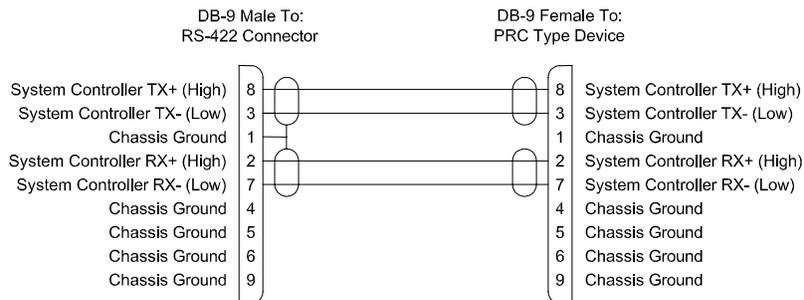
**Figure 7. RS-422 Serial Cable**
