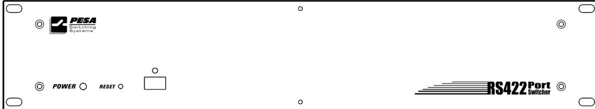
Figure 13. RS-422 Port Switcher Front View
