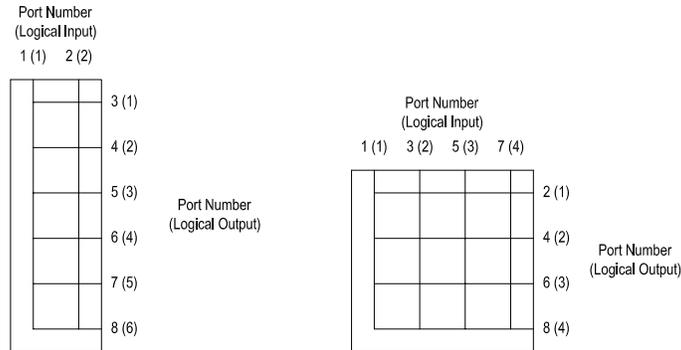
Figure 16. Sample Port Allocation for 8-Port Switcher
