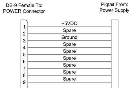
**Figure 11. Power Supply Pigtail**
