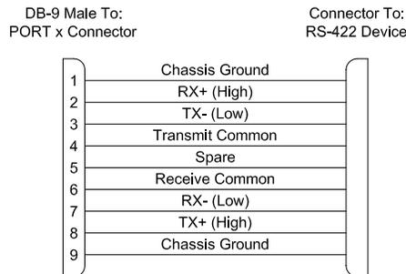
Figure 3. RS-422 Device Cable
